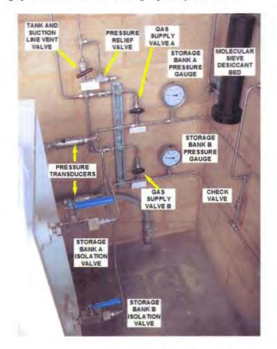
Figure 2. Gas supply plumbing
