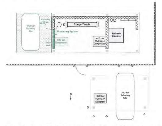
Figure 1. Plan view of Station Layout showing station modifications in green
