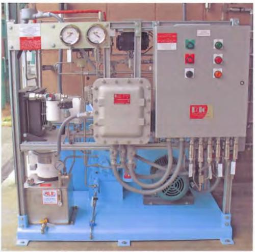
Figure 3: 700 bar hydrogen compressor
