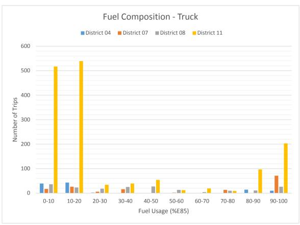
Figure 6.22. Fuel composition histogram for trucks operating in the demonstration program.
