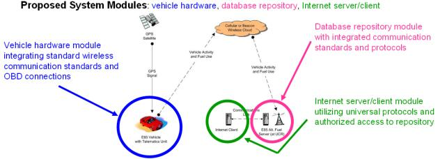
Figure 7.1. Proposed architecture for future deployment.
