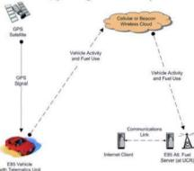
Figure 1 Caltrans E85 Monitoring System Architecture.
