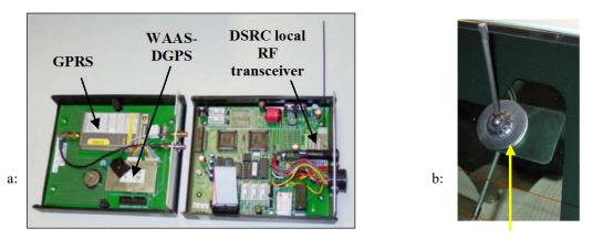
**Figure 2.2. a)** On-Board Telematics Hardware: GPRS - General Packet Radio Service cellular modem; WAAS-DGPS – Wide Area Augmentation System enabled Differential Global Position System receiver; DSRC – Dedicated Short Range Communications. **b)** Dual GPRS/GPS antenna.
