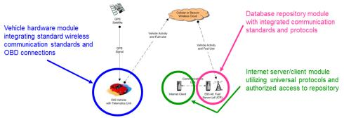
Figure ES.1. E85 alt-fuel system monitoring architecture with combined cellular and Wi-Fi.
