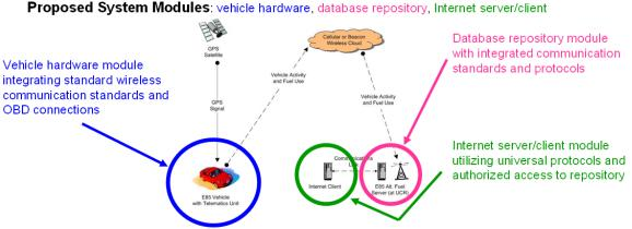
Figure 2. Proposed architecture for future deployment.
