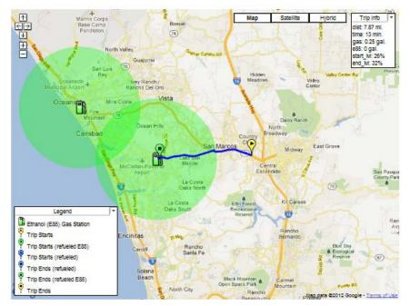
Figure ES.2. Caltrans E85 user interface mapping function.
