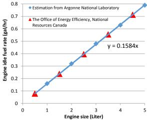
Figure 4.18 – Idle fuel rate vs. engine size
