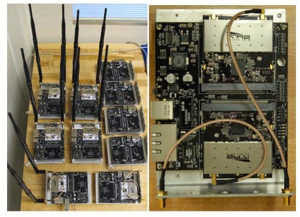
Figure 4.6 AHMCT 5.8 GHz mesh network experiment setup
