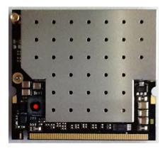
Figure 4.5 4.9 GHz wireless radio (www.doodlelabs.com)
