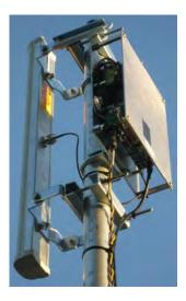
Figure 4.4 AHMCT 5.8 GHz point-to-point communication experimental setup
