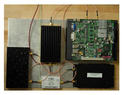
Figure 4.1 OpenBTS base station hardware implementation at AHMCT
