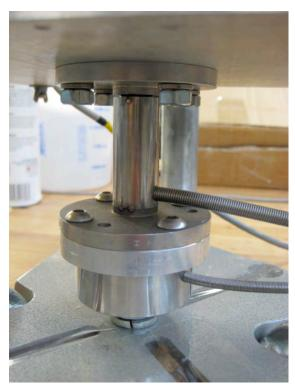
Figure 3-9: Torque cell and load cell affixed between test bed and stand
