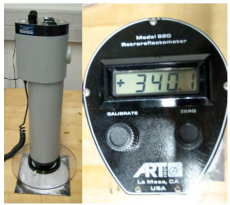
Figure 3-16: Retroreflectometer; Detail of calibration knobs and readout
