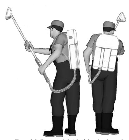
Figure 2-2: Conceptual sketch of sign cleaning tool
