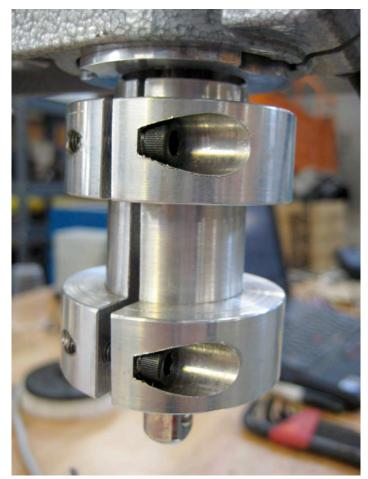
Figure 3-6: Coupling from shaft to brush
