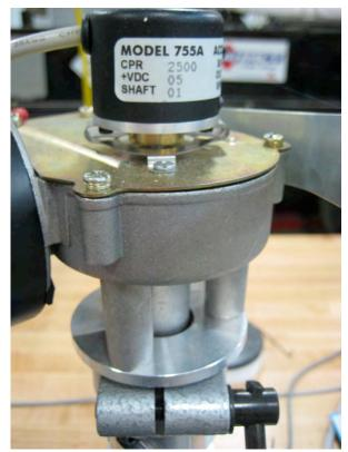
Figure 3-14: Encoder attached to back of motor
