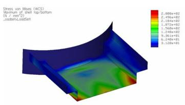
Figure 6.2 Result From Finite Element Analysis on Skid Plate with No Gussets
