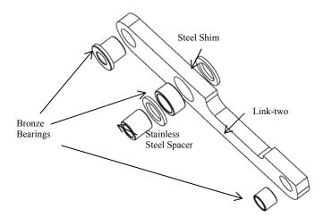
Figure 5.17 Link-three Sub-assembly
