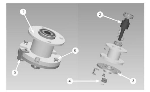
Figure 4.21 Adaptor Cup Assembly components of interest: 1) Bearing Cup, 2) Power Shaft, 3) Adaptor Plate, 4) cutter pinion, 5) HT-Bracket, 6) HT-thumb screw (X2)
