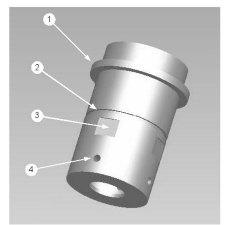
Figure 4.28 RHT-Bearing Carrier selected details: 1) BC-lip, 2) BC-snap ring groove, 3) BC-flat (X2), and 4) BC-machine screw hole (X4).
