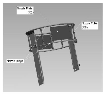
Figure 4.15 New Nozzle Bracket components.
