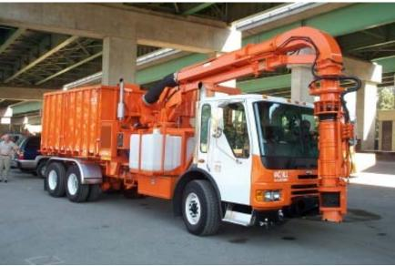
Figure 1.1 ARDVAC Attached to Boom Vacuum Truck
