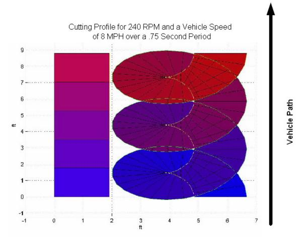
Figure 4.12 cutter profile for intermittent vegetation.
