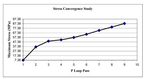
Figure 6.7 Max Stress Convergence for Aluminum Bracket with no Fillet
