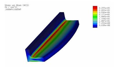
Figure 6.6 Result from Finite Element Analysis on Steel Bracket with Fillet and Thicker Flange
