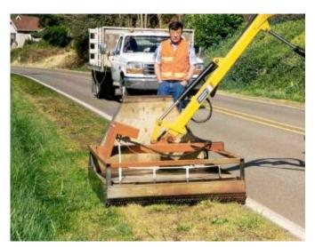
Figure 2.7 Infrared vegetation control unit
