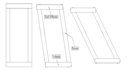
Figure 3.6 Parallelogram maintains constant forward sweeping orientation.
