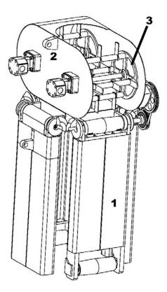
Figure 8.2 Tumbleweed Machine - 1) Arms, 2) Housing, & 3) Cutter Assembly
