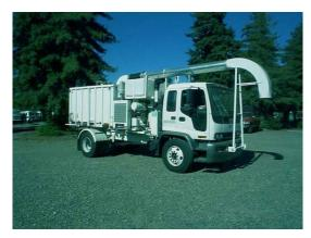
Figure 3.2 Fixed boom vacuum vehicle.
