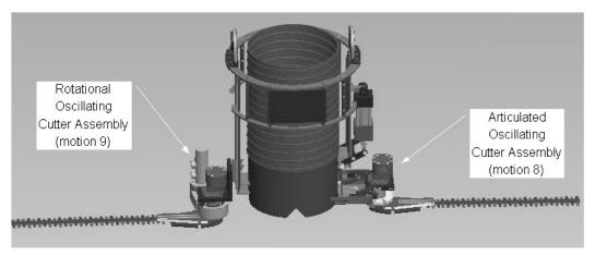
Figure 4.16 Oscillating Cutter Assembly locations.
