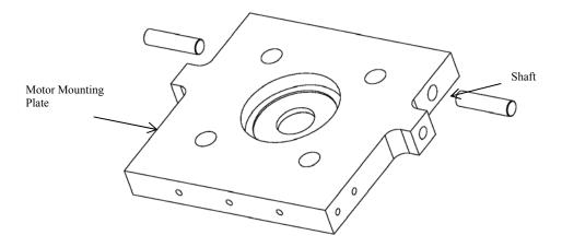
Figure 5.15 Articulating Motor Plate Sub-assembly
