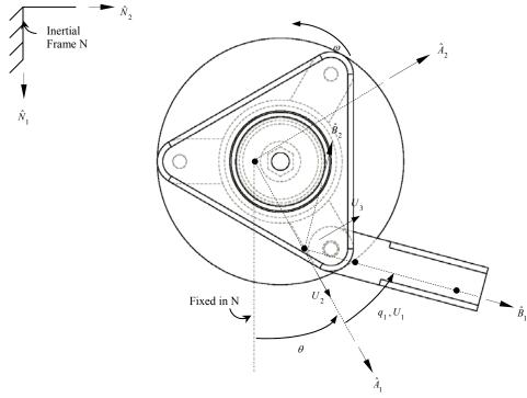
Figure 7.3 Reference Frames and Generalized Coordinates and Speeds
