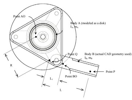
Figure 7.4 Geometry for Dynamic Model
