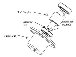
Figure 5.13 Bearing Carrier Sub-assembly
