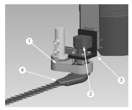
Figure 4.22 Selected Rotational Oscillating Cutter Assembly components: 1) RHT-Belt Drive Assembly (shrouding), 2) cutter motor, 3) RHT-Motor Mounting Plate, and 4) hedge trimmer base configuration
