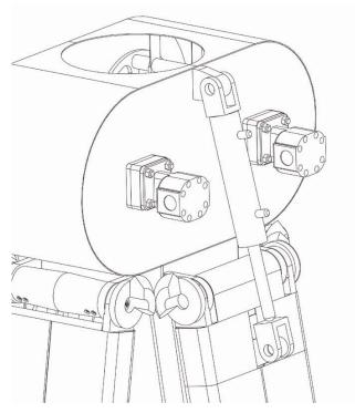
Figure 8.20 Actuating Cylinder
