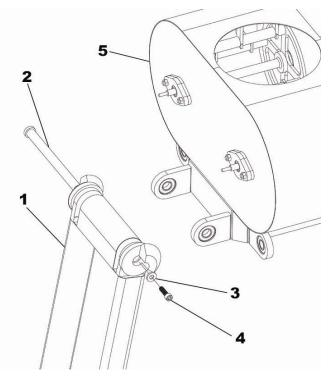
Figure 8.15 Bare Arm Connection: 1) Arm, 2) Arm Shaft, 3) Restraining Washer, 4) Retaining Screw, & 5) Housing.
