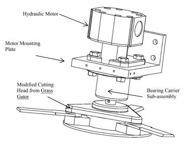
Figure 5.12 Stationary Cutter Sub-assembly
