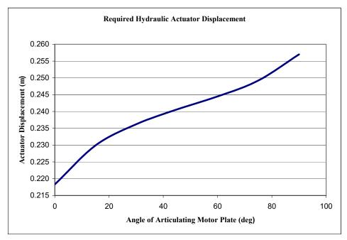
Figure 5.4 Required Actuator Displacement for Full Motor Plate Articulation
