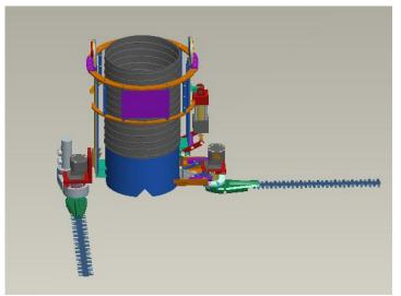
Figure 1.8 Hedge Trimmer Cutting Fixture
