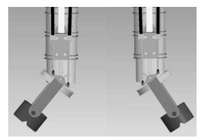
Figure 3.13 Motion 7 due to Long Cylinders applying torque through the Cylinder Pivot Flange.
