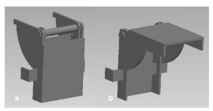
Figure 4.23 RHT-hinge close up (fastener holes not shown). a) closed, b) opened.
