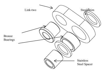
Figure 5.16 Link-two Sub-assembly
