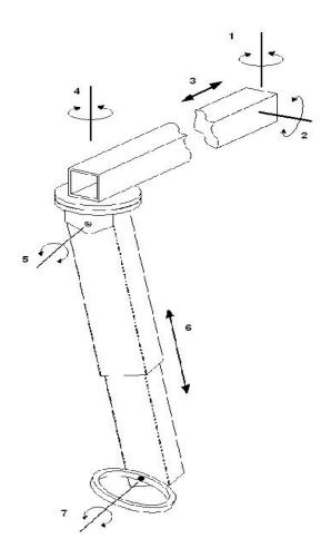
Figure 3.5 Initial end-effector motion
