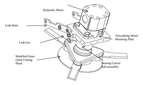
Figure 5.14 Articulating Cutter Sub-assembly
