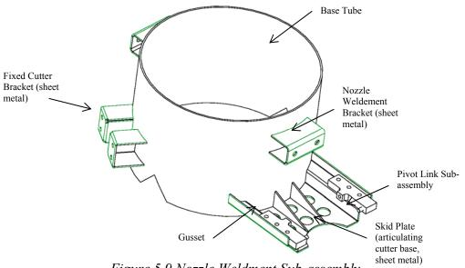
Figure 5.9 Nozzle Weldment Sub-assembly
