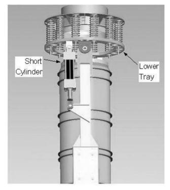
Figure 3.8 CAD model of the upper portion of the end-effector.
