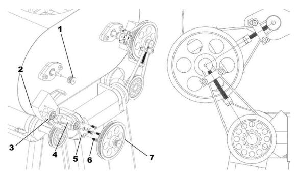
Figure 8.18 Left: Installation of pulley system: 1) 11-Tooth Pulley, 2) Composite Pulley Housing, 3) Composit Pulley Bearing, 4) Composite Pulley Shaft, 5) Pulley Housing Cover, 6) Pulley Housing Cover Screw, & 7) Composite Pulley (11 & 72 Tooth Pulleys). Right: Frontal view of pulley system.
