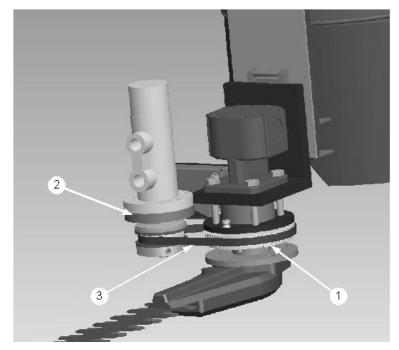
Figure 4.25 RHT-Belt Drive components with the shrouding removed: 1) RHT-Rotary Adaptor Assembly, 2) rotary motor assembly, and 3) neoprene timing belt.
