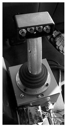
Figure 3.15 Three-axis joystick controlling motions 5-7
