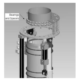
Figure 3.7 Cutaway of ball bearing joint for motion 4
