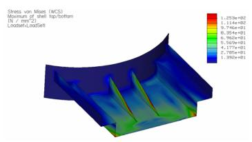
Figure 6.1 Result from Finite Element Analysis on Skid Plate with Gussets
