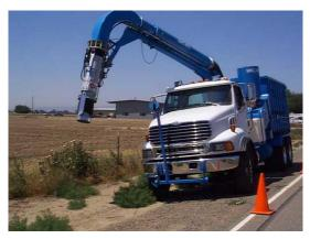
Figure 3.3 Industrial vacuum vehicle with articulated boom.
