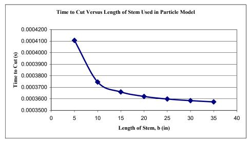
Figure 7.5 Cutting Time versus Length of Stem Being Cut
