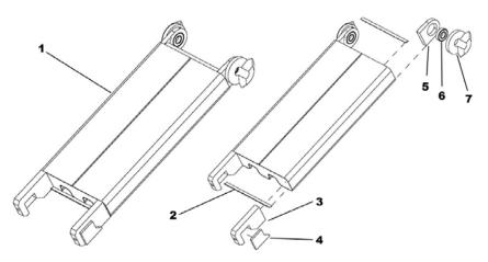
Figure 8.9 Conveyor Belt Arm: an unassembled arm is on the left, and to the right is an exploded view of the unassembled arm. 1) Arm Frame, 2) Belt Scoop, 3) Tension Bracket, 4) Bracket Stiffener Plate, 5) Pillow Block, 6) Arm Bearing, & 7) Mitre Gear
