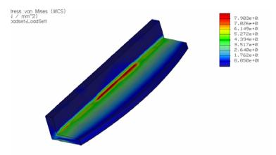
Figure 6.5 Result from Finite Element Analysis on Aluminum Bracket with No Flange nor Fillet
