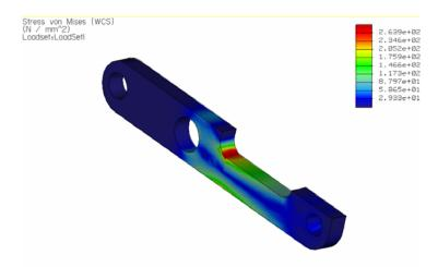
Figure 6.9 Result from Finite Element Analysis on Link-three
