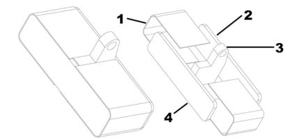
Figure 8.12 Cylinder Mount Section: 1) Cylinder Block Cover, 2) Lower Cylinder End Cap, 3) Cylinder Mount, & 4) Upper Cylinder End Cap
