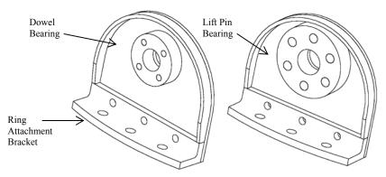
Figure 5.6 Upper Attachment Plate Sub-assemblies
