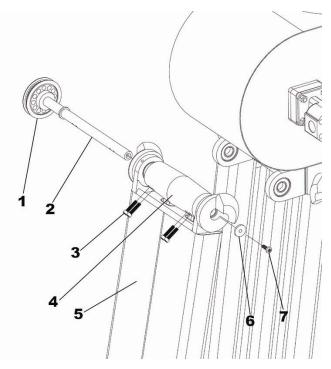
Figure 8.16 Conveyor Belt Arm Installation: 1) Conveyor Drive Pulley, 2) Pulley Drive Shaft, 3) Pulley Screws, 4) Drive Pulley, 5) Conveyor Arm, 6) Washer, & 7) Screw. Not shown: Conveyor Belt.
