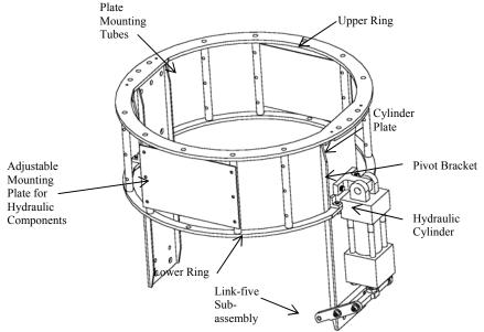
Figure 5.7 Hydraulic Mounting Cage Sub-assembly
