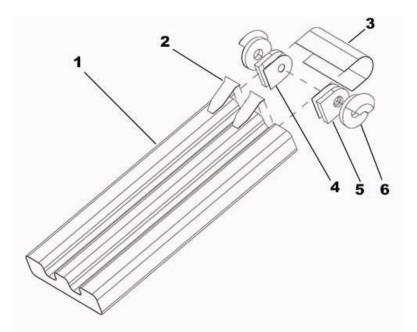
Figure 8.11 Non-actuating Bare Arm: 1) Arm Frame, 2) Gap Angle, 3) Gap Blocker, 4) Gap Blocker Side, 5) Shaft Block, & 6) Bevel Gear.
