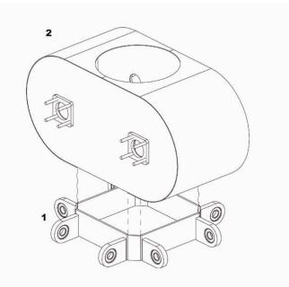
Figure 8.5 Housing assembly: 1) arm mounting ring & 2) cutter housing
