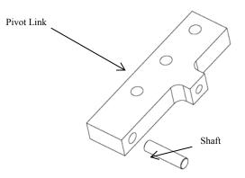
Figure 5.10 Pivot Link Sub-assembly
