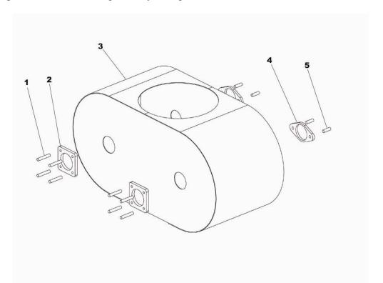
Figure 8.6 Cutter Housing: 1) Motor Mount, 2) Motor Mount Boss Plate, 3) Cutter Housing, 4) Pulley Mount Boss Plate, & 5) Pulley Mounts
