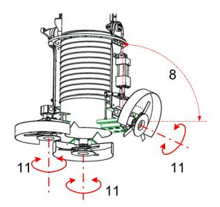
Figure 4.6 Motions 8 and 11 of the rotary cutter system.
