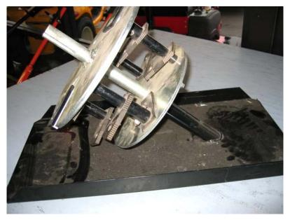
Figure 8.1 Cutting wheel from a commercial Chipper/Shredder
