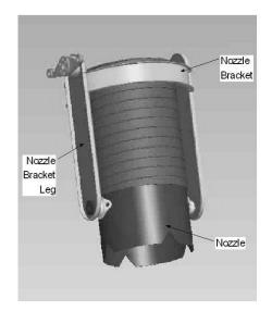
Figure 3.11 Original Nozzle assembly.
