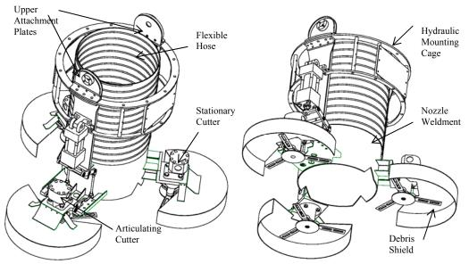
Figure 5.1 Rotary Impact Cutting Fixture Final Assembly
