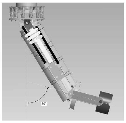
Figure 3.14 Extreme Nozzle positioning.
