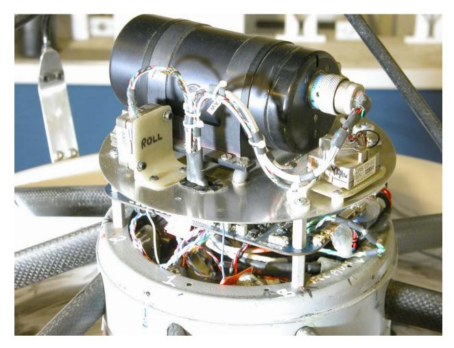
The sensor signals are passed through low-pass filters before entering the micro controller to reduce the effects of high frequency noise that could provide a false signal down into the control system bandwidth due to the limited sampling rate of the micro controller.
