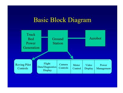
Ground Control Station Block Diagram
