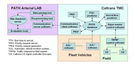
Figure 5-2 ATSP System Software Architecture
