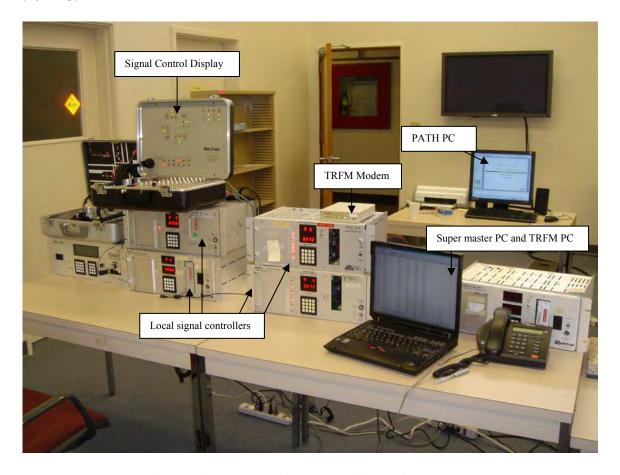
Figure 5-3 Hardware-in-the-loop Simulation Test-bed
