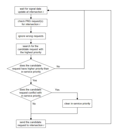
Figure 1-2 Flow Chart of TSP Algorithm
