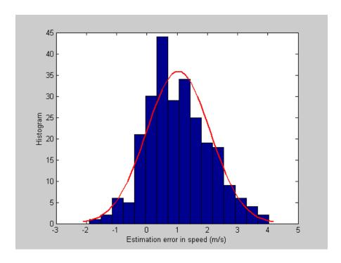
Figure 2-7 Histogram of Speed Estimation Error by Equation 2-3
