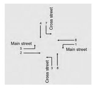
Figure 4-1 Definitions of standard NEMA 8 movements
