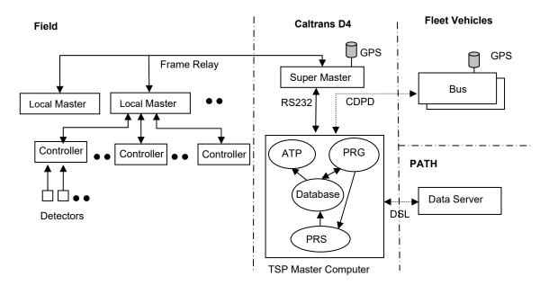
Figure 1-1 System Architecture of the Prototype ATSP System
