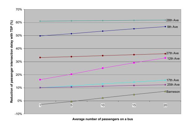
Figure 6-5 Sensitivity analysis of passenger delay reduction (%)
