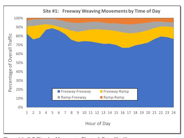
Figure 4.4 O-D Weaving Movements--Bluetooth Data -Site #1
