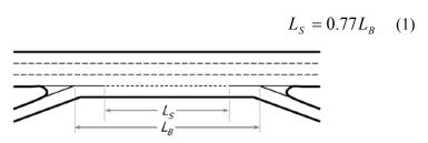
Figure 2.2 Weaving Section Length (source: Exhibit 12-2, HCM2010)
