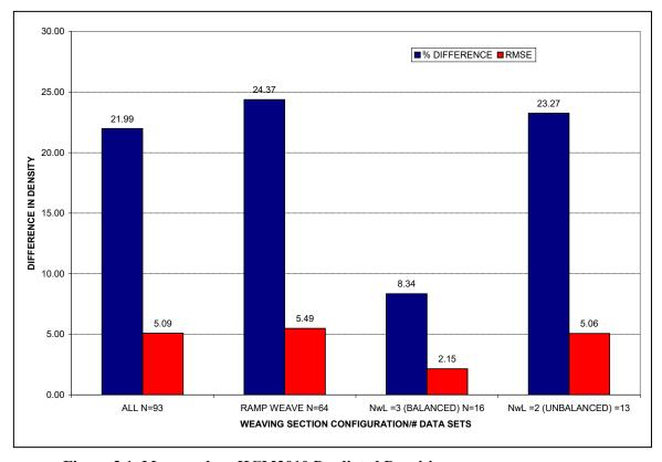
Figure 3.1 Measured vs. HCM2010 Predicted Densities
