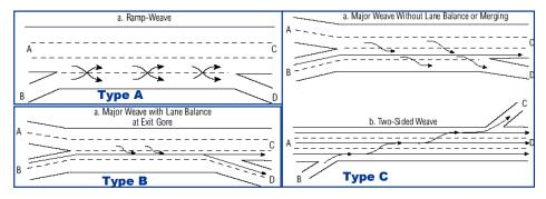
Figure 2.1 Configurations of Freeway Weaving Sections (HCM2000/1985)
