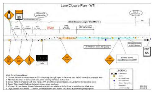
Figure 5: sDrum System Deployment – Modified Caltrans Image
