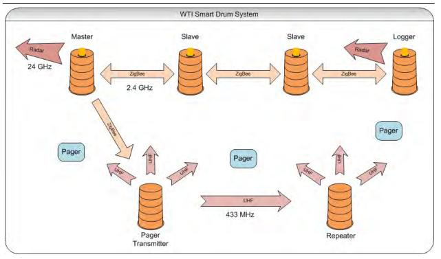
Figure 2: sDrum System Architecture
