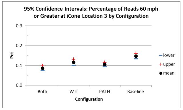
Figure 8: Confidence Interval Plots for Hourly Percentage of Reads 60 mph or Greater Measured by iCones by Configuration at iCone Location 3
