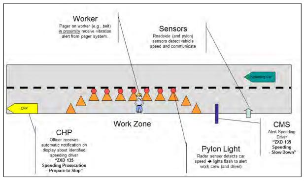
Figure 1: aSE System Diagram
