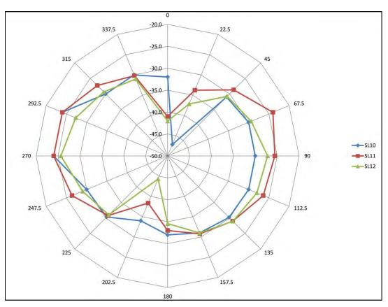
Figure 9: XBee Radio Antenna Patterns
