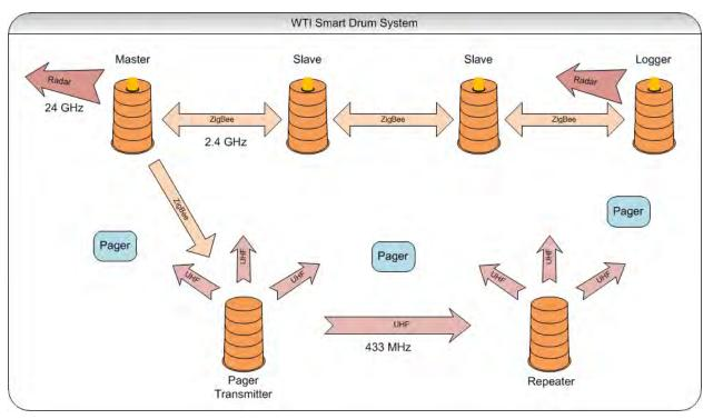
Figure 2: sDrum System Architecture
