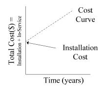
Figure 2 Installation cost relative to life-cycle cost
