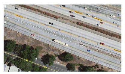
Figure 9: Shows the attenuator's location and the associated virtual gore point. The virtual gore point is the point where the lane lines diverge to direct traffic. The term "virtual" is used since there is no physical barrier.
