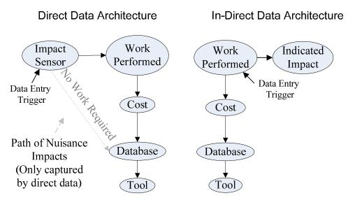
Figure 14: Data flow of direct data vs. indirect data
