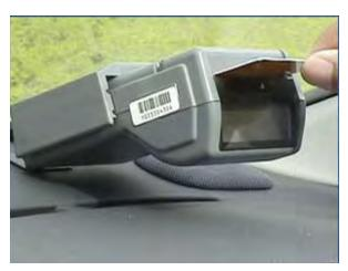
Figure 4: Transponder and Smart Card (EPVIS 2002)
