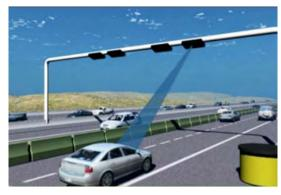
Figure 2: Roadside antenna communicates with vehicle-mounted transponder via DSRC (TransNet 2008)
