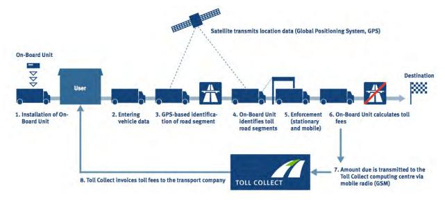
Figure 5: German Toll Collect Technological Configuration (Toll Collect 2007)
