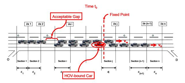
Figure 3-4. Acceptable Gap at time  $t = t_0$
