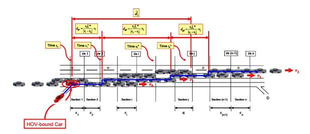
Figure 3-9. Four-lane freeway example of Acceptable Gap conditions relative to unsuccessfully accessing preferred Ingress/Egress point i/e *i*
