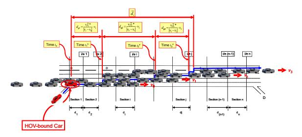
Figure 3-8. Four-lane freeway example of Acceptable Gap conditions relative to successfully accessing preferred Ingress/Egress point i/e i
