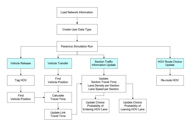
Figure 4-1. Paramics buffer-separated HOV access API Schematic
