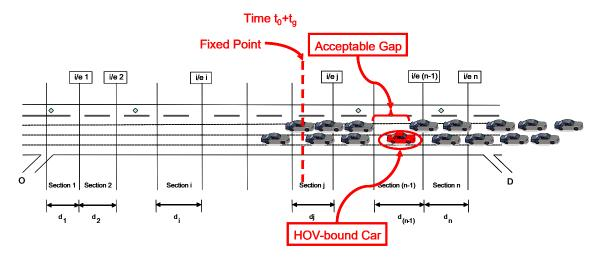
Figure 3-6. Acceptable Gap at time  $t = t_0 + t_g$
