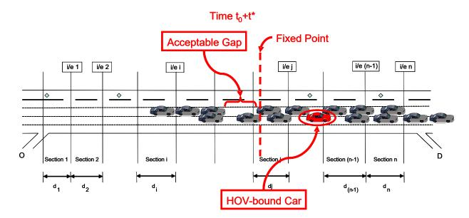
Figure 3-5. Acceptable Gap at time  $t = t_0 + t^*$
