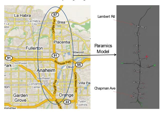
Figure 5-19. Freeway Network for Sensitivity Analysis: SR-57 Network
