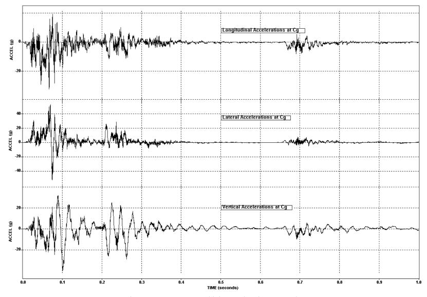
Figure 6-4 – Test 601 Vehicle Accelerations -Vs- Time
