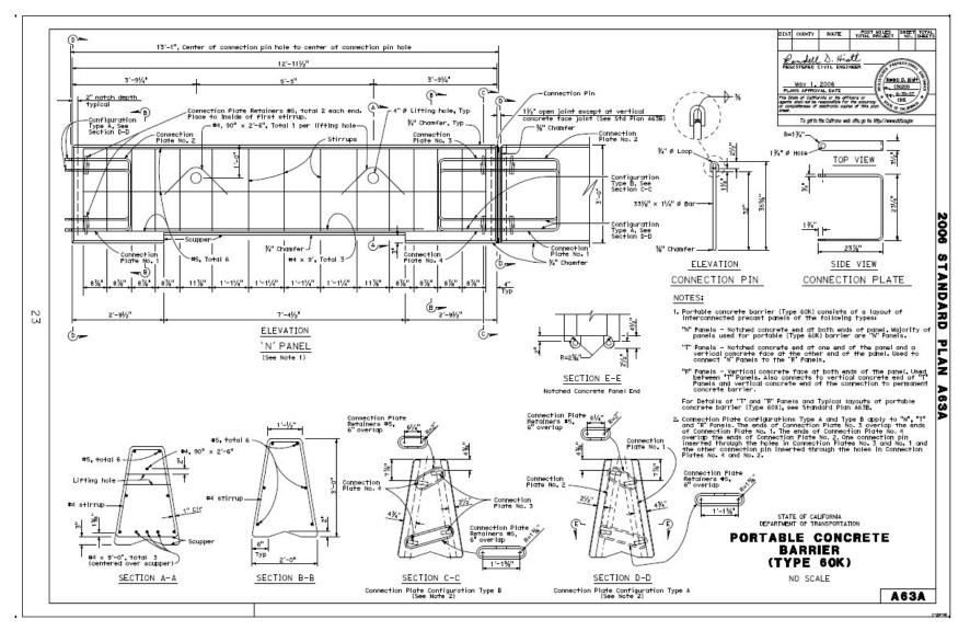
Figure 6-8 – Type 60 Standard Plan
