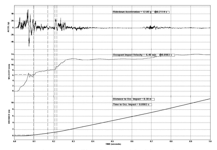
Figure 6-6 – Test 601 Vehicle Lateral Acceleration, Velocity and Distance -Vs- Time
