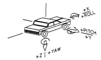
Figure 6-3 – Vehicle Accelerometer Sign Convention
