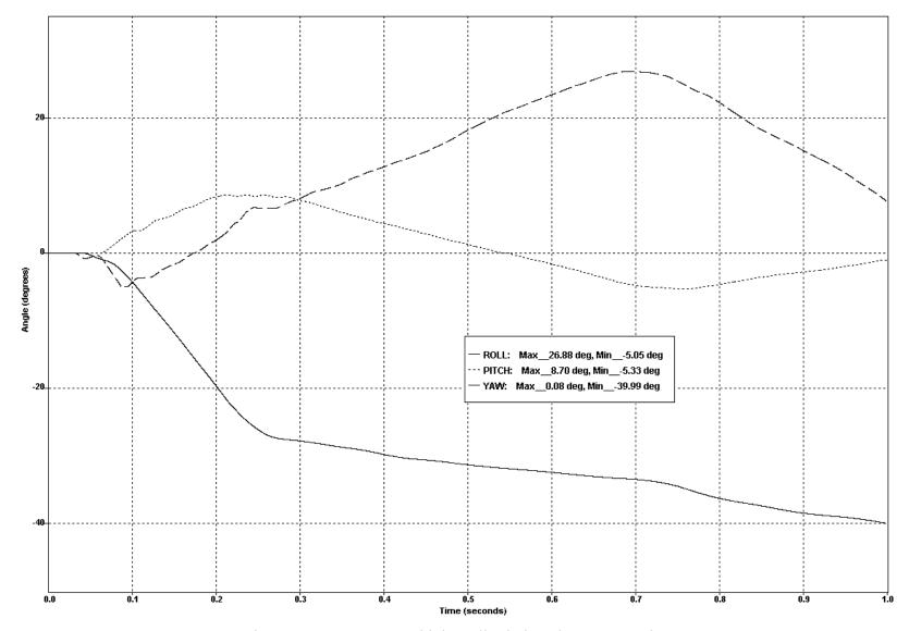
Figure 6-7 – Test 601 Vehicle Roll, Pitch and Yaw -Vs- Time
