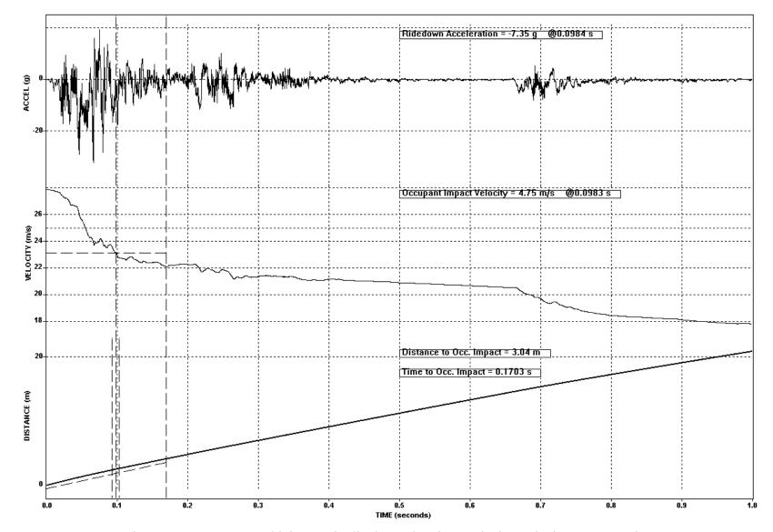
Figure 6-5 – Test 601 Vehicle Longitudinal Acceleration, Velocity and Distance -Vs- Time
