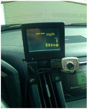
Figure 12: CACC display (right of steering wheel)
