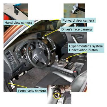
Figure 17: Vehicle Interior, Showing Locations of Video Cameras
