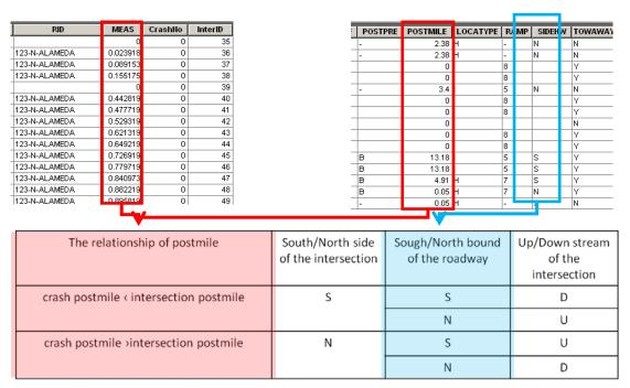
Figure 5. Technique to Identify Upstream and Downstream Crashes
