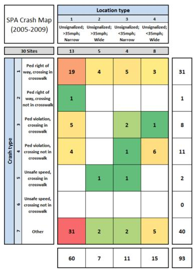
Figure 13. Systemic Hot Spots Identification Matrix for Road Segments
