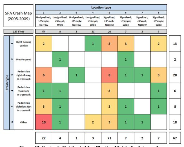
Figure 12. Systemic Hot Spots Identification Matrix for Intersections
