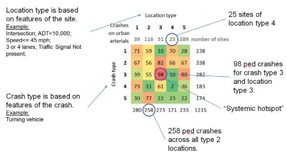
Figure 9. Example of the Systemic Hot Spot Identification Matrix
