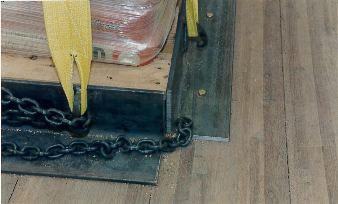
Figure 2.27 - 150 mm Angle Irons Were Used To Constrain The Pallets Of Sand for Test 513
