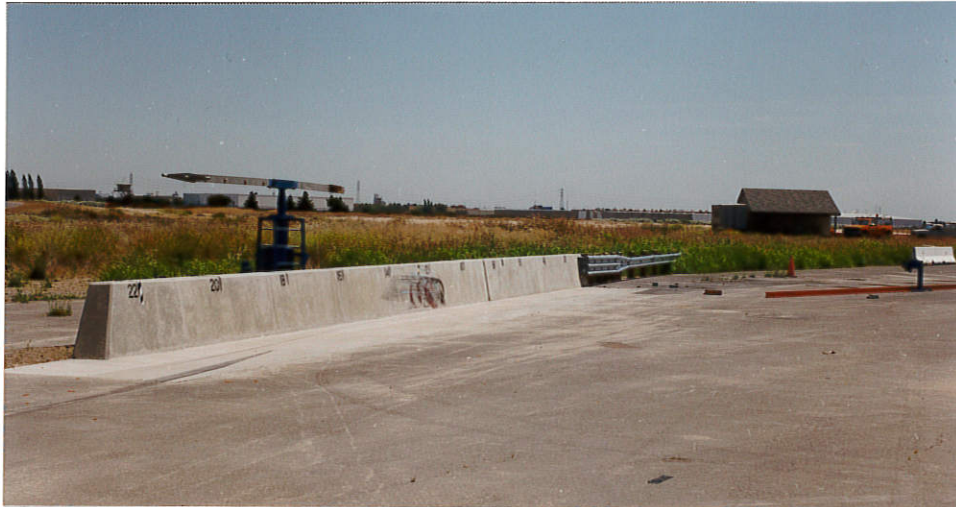
Figure 2.14 - Type 70 Barrier Prior To Test 512
