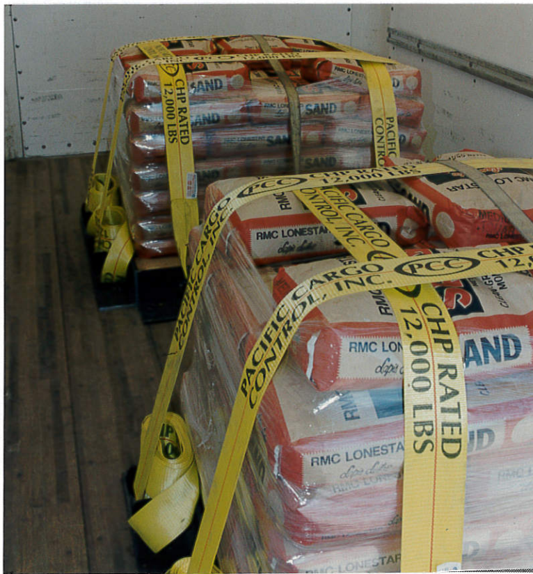
Figure 2.26 - Two Pallets Of Sand Used For Ballast on Test 513
