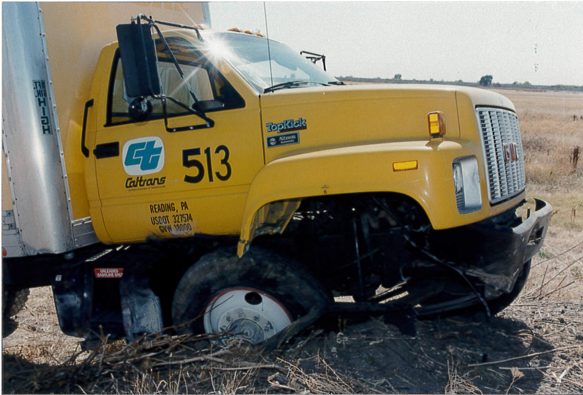
Figure 2.32 - Right Side Of Cab For Test 513 After Test
