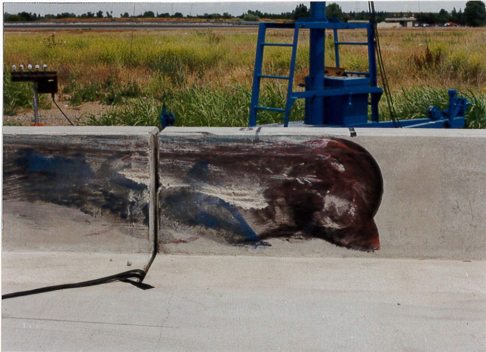
Figure 2.19 - Scuff Marks on Barrier for Test 512
