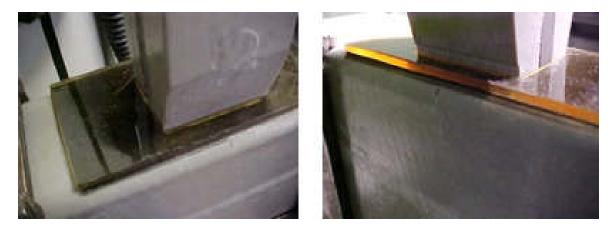
Figure 36 Photostress method Applied to Composite Snap-Fit
