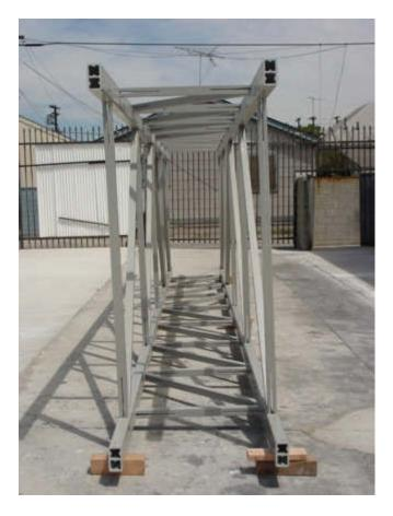
Figure 25 Assembled Overhead Sign Structure
