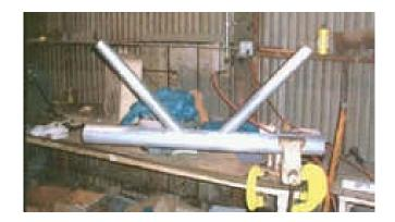
Figure 2 Weld Fatigue Failure in Aluminum Sign Bridge as Experienced by NYDOT.
