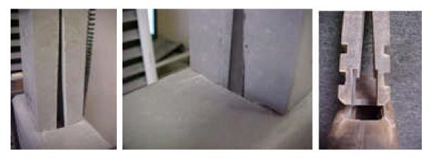
(b) Figure 41 First cracks observed in the Snap-Fit
