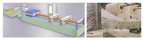
Figure 18 Fabrication of Sign Truss Elements by Pultrusion Process
