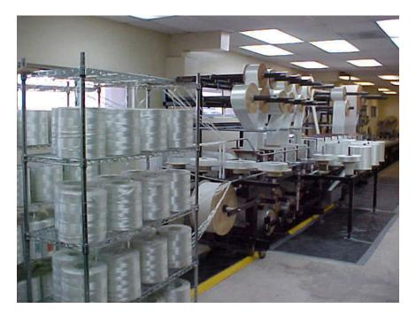
Figure 20 Global view of the Pultrusion Setup
