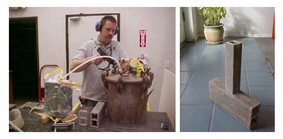
Figure 16 a, b Snap-joint infusion and finished snap joint assembly
