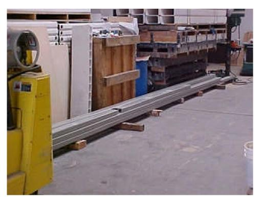
Figure 23 Finished Pultrusions
