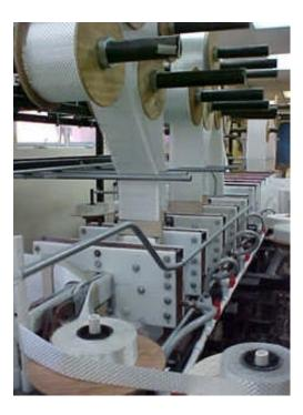
Figure 21 Detail of fiber Dispensing
