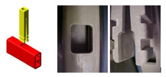
Figure 43 Snap-fit Geometry change for increased load capacity
