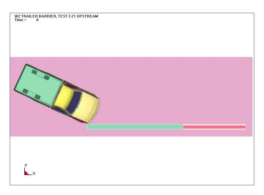
Figure 7-13 Initial Orientation in Plan View for the Upstream Impact Simulation
