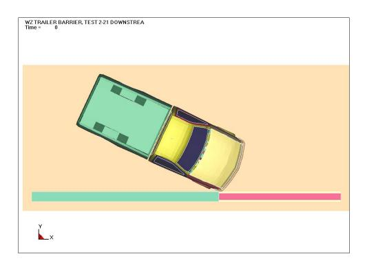
Figure 7-17 Initial Orientation in Plan View for the Downstream Impact Simulation
