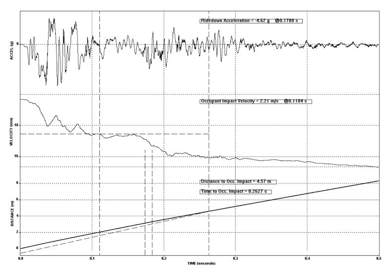
Figure 7-5 Test 641 Vehicle Longitudinal Acceleration, Velocity, and Distance -Vs- Time
