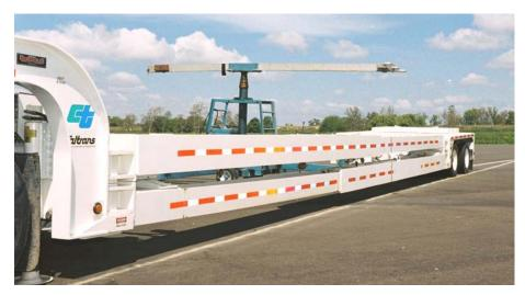
Figure 2-11 Trailer in Barrier Mode for Test 641
