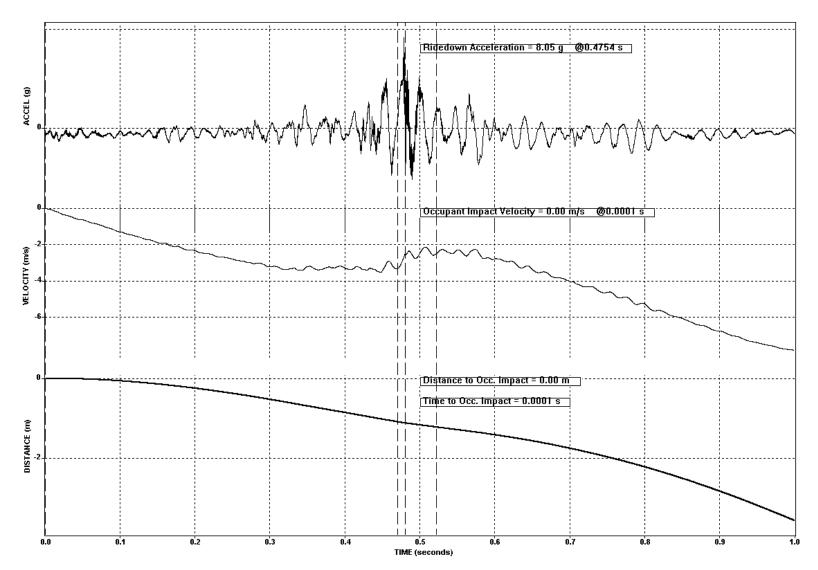
Figure 7-9 Test 641 Second Impact Vehicle Lateral Acceleration, Velocity, and Distance -Vs- Time
