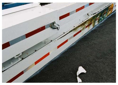
Figure 2-17 Barrier After Test 641
