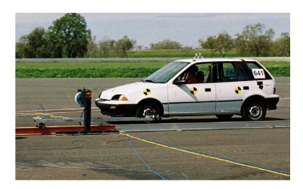
Figure 7-1 Vehicle Guidance System
