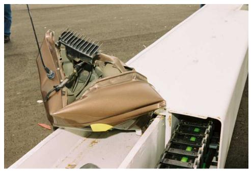
Figure 2-31 Close-up of the Vehicle's Sheet Metal in Test 642
