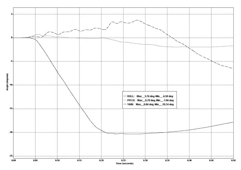
Figure 7-7 Test 641 Vehicle Roll, Pitch, and Yaw -Vs- Time
