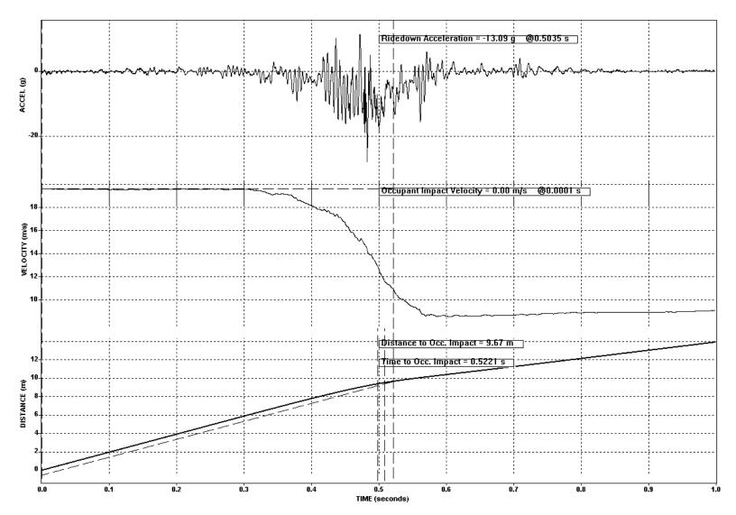
Figure 7-8 Test 641 Second Impact Vehicle Longitudinal Acceleration, Velocity, and Distance -Vs- Time
