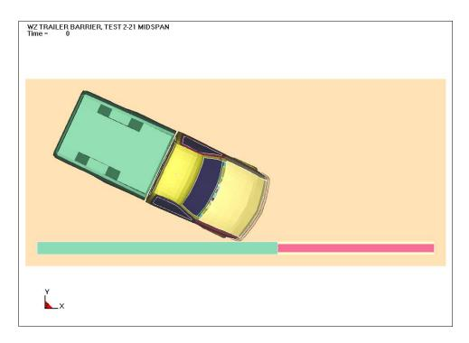
Figure 7-15 Initial Orientation in Plan View for the Mid-Span Impact Simulation
