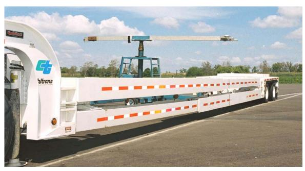
Figure 2-6 Fully Deployed Balsi Beam
