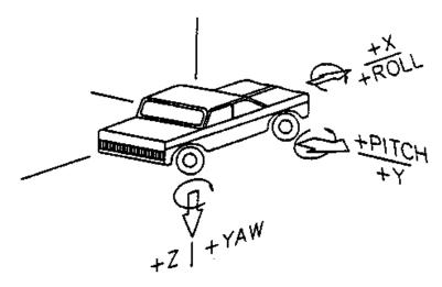
Figure 7-3 Vehicle Accelerometer Sign Convention
