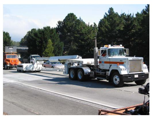
Figure 2-4 Balsi Beam Deployment 4
