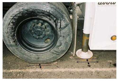
Figure 2-32 Trailer Tire and Brace Displacement in Test 642
