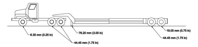
Figure 2-21 Later Displacement of the Tractor Truck and Trailer to Test 642
