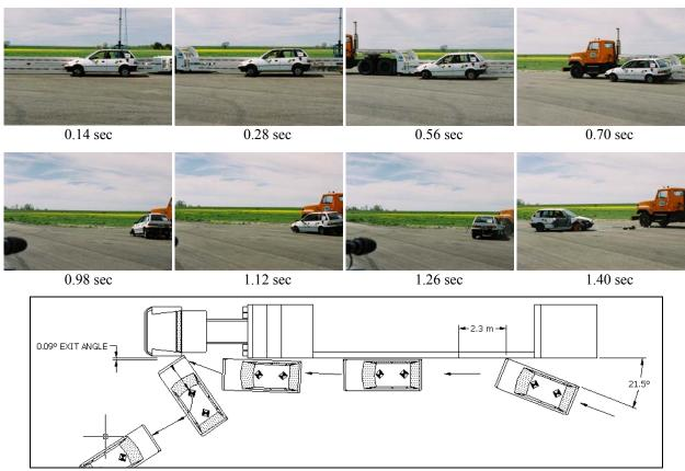
Figure 2-20 Test 641 Impact Sequence and Diagram
