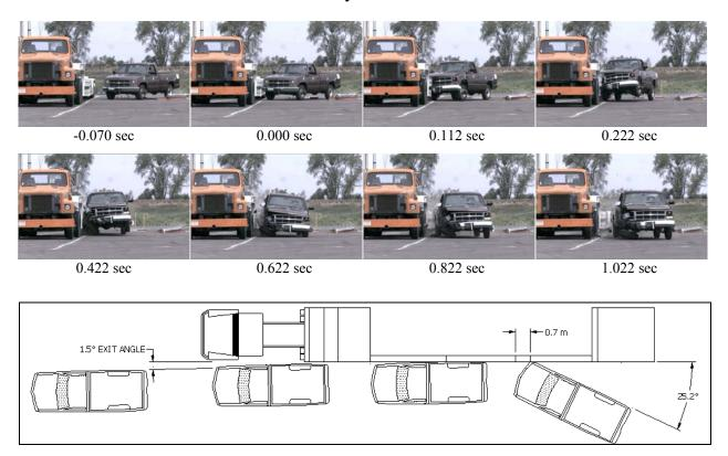
Figure 2-33 Test 642 Impact Sequence and Diagram
