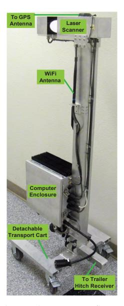
Figure 3.1: The second-generation profle sensing system.
