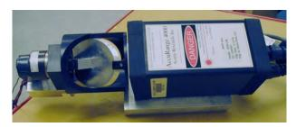
Figure 3.3: The scanning laser rangefnder.
