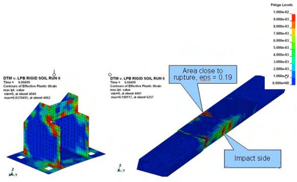
Figure 11. Impact side and Area close to rupture
