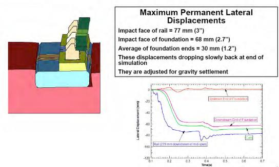
Figure 15. Maximum Permanent Lateral Displacements
