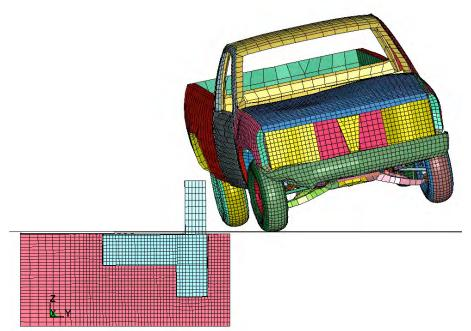
Figure 8. C2500 Pickup Impact on Cross-Section 9
