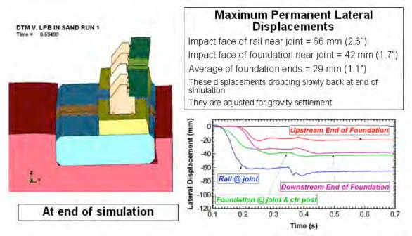
Figure 12. Maximum Permanent Lateral Displacements
