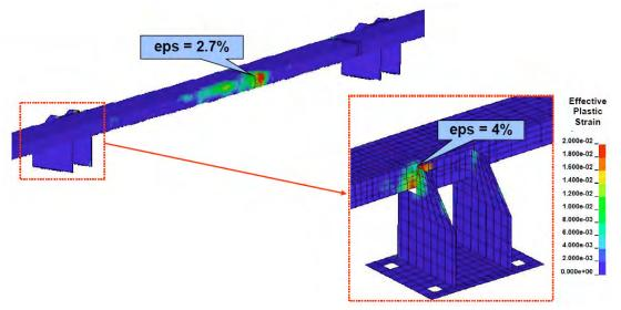
Figure 14. Plastic Strains at Mid-Span
