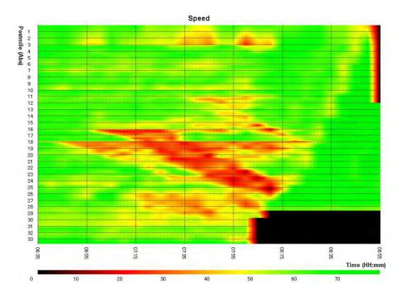
Figure 16-9: Speed contour for I-880: Incident and 20% diversion and familiarity 25
