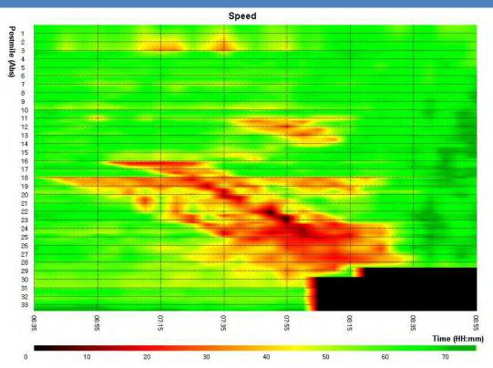
Figure 16-1: Speed contour for I-880: Incident and 10% diversion
