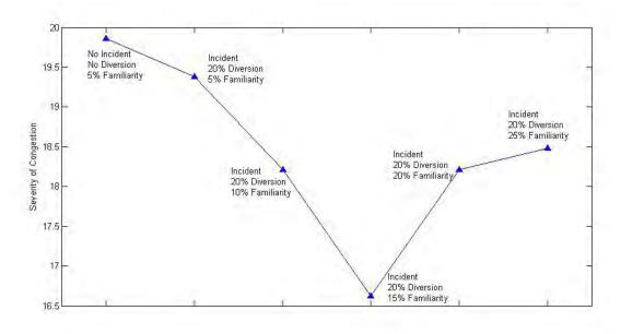
Figure 9-22: Severity of congestion for different QID levels
