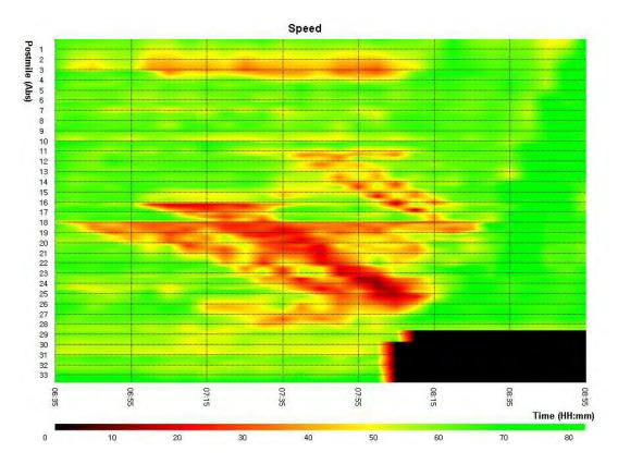
Figure 9-20: Speed contour for I-880, Scenario 5: Incident and 20% diversion and 20% QID
