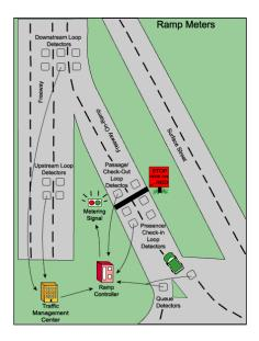
Figure 13-7. Ramp metering diagram ci
