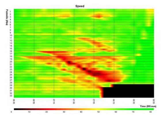
Figure 16-6: Speed contour for I-880: Incident and 20% diversion and familiarity 10
