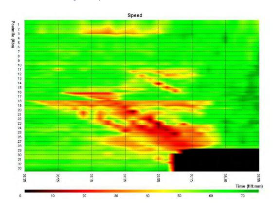
Figure 16-2: Speed contour for I-880: Incident and 20% diversion
