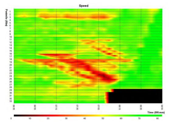
Figure 16-8: Speed contour for I-880: incident and 20% diversion and familiarity 20
