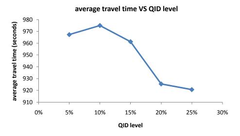
Figure 9-12: Average travel time for different QID levels
