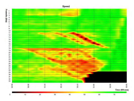
Figure 9-16: Speed contour for I-880, Scenario 1: No incident
