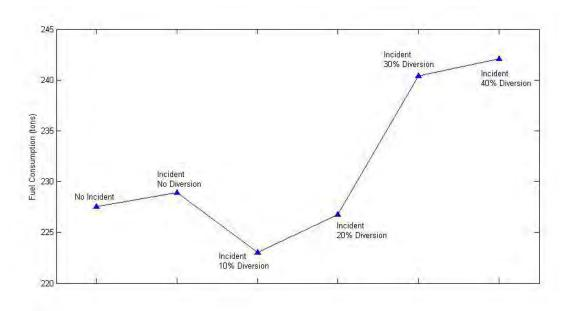
Figure 9-25: Fuel consumption for different CMS diversion rate
