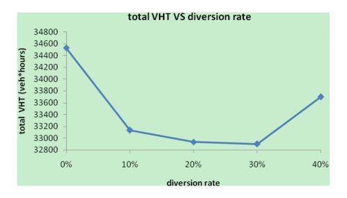
Figure 9-11: Total VHT under different diversion rates
