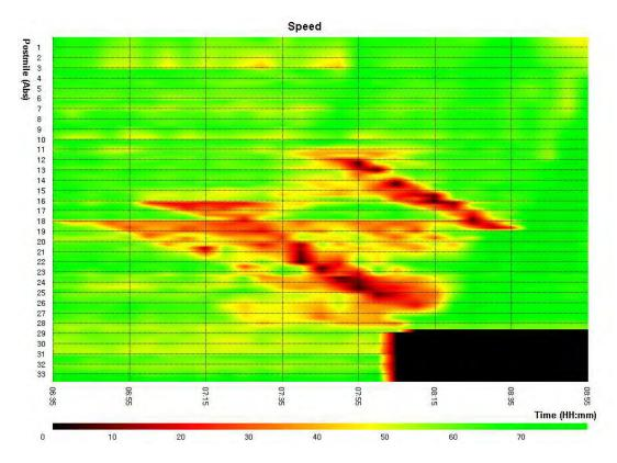
Figure 16-7: Speed contour for I-880: Incident and 20% diversion and familiarity 15
