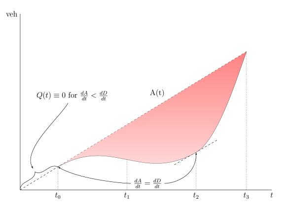
Figure 3.14: The formation of a queuing for a typical incident
