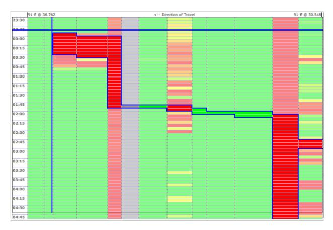
Figure 3.12: A case where distance weighting is helpful. In this plot, traffic travels from the top right corner to the bottom left. The incident occurred where the two blue lines cross. The small congestion plume adjacent to the cross is the appropriate extent of impact. However, the algorithm attaches the unrelated upstream congestion because the resulting false positives don't outweigh the addition of new correct positives.
