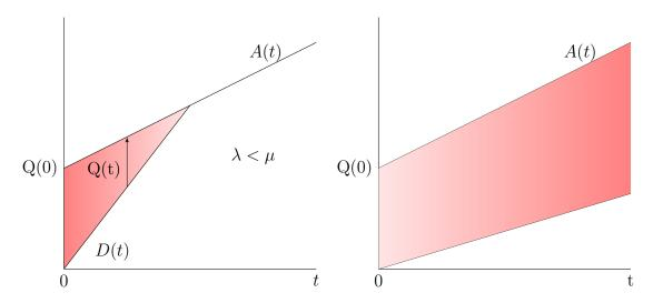
Figure 3.13: Queuing under constant arrival and service rates. In both figures, a queue of length Q(0) exists at time 0 and there is some constant arrival rate  $A(t) = \lambda$ . The figure on the left shows the dissipation of the queue when the arrival rate is less than the service rate  $\lambda < \mu$ . The figure on the right shows the increasing queue caused by the oversaturated conditions  $\lambda > \mu$ .
