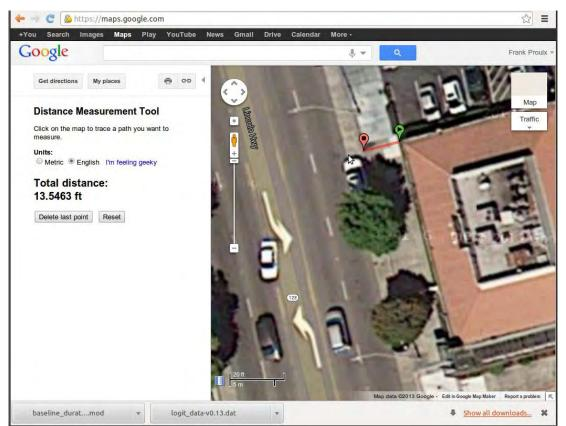
Figure 14. Screenshot Showing How to Measure the Width
