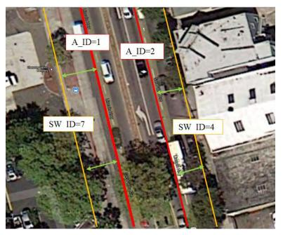
Figure 12. Example of Sidewalk Labeling
