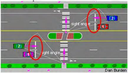
Figure 29. Example of "Advanced Stop Bars" (Source: saferoutesinfo.org)
