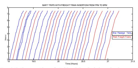
Figure 3-12: Time Space Diagram for Freight train insertion in the evening slots
