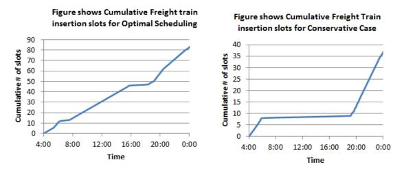
Figure 3-13. Cumulative Freight Train insertion slots (Left), Optimal Scheduling (Right): Conservative case
