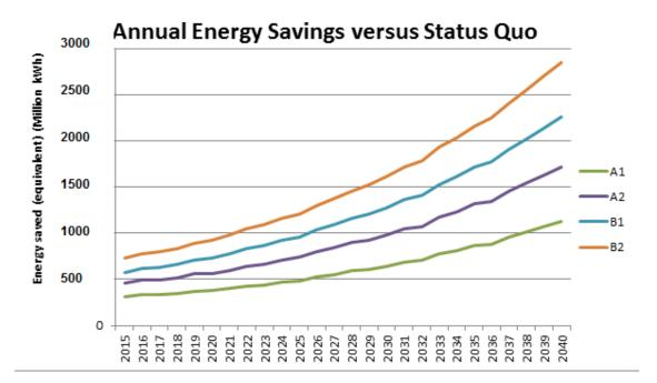
Figure 4-10. Predicted energy (kw/h) saving vs. Status Quo for the 4 alternatives
