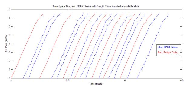
Figure 3-11: Time Space Diagram showing Freight train insertion in the morning slots
