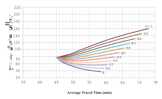
Figure 4.6 Change in total emissions with travel time as LOS is reduced for bus (scenario 2)
