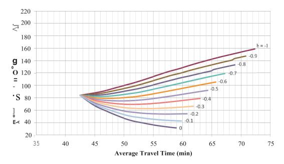
Figure 4.8 Change in total emissions with travel time as LOS is reduced for LRT (scenario 2)
