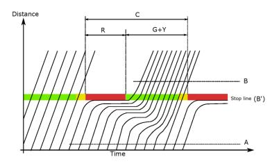
Figure 2. Distance-time diagram for a signalized intersection.
