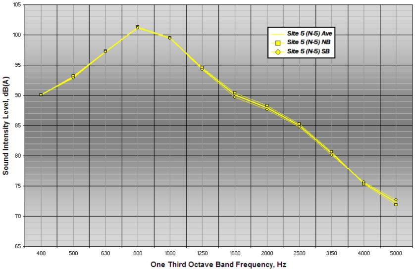
Figure A5. One-Third Octave Band Levels for Site 5 (N-5), Burlap Drag PCC Pavement in NB & SB Directions
