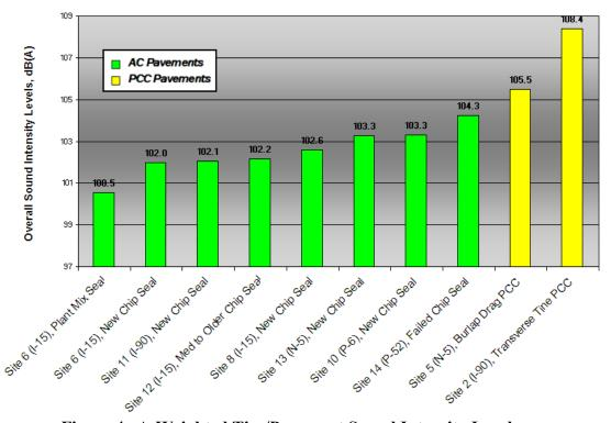
Figure 4. A-Weighted Tire/Pavement Sound Intensity Levels
