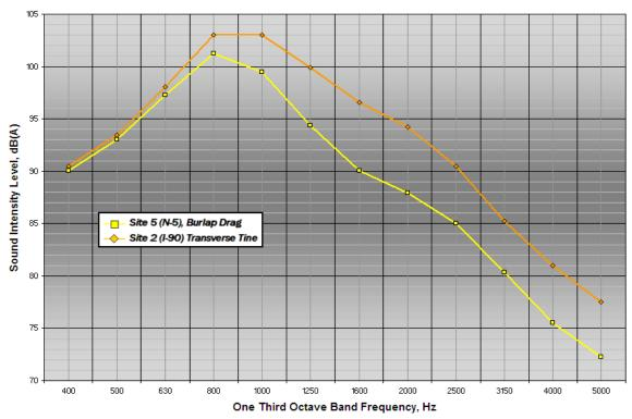
Figure 7. One-Third Octave Band Levels for PCC Pavements
