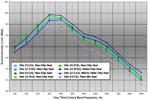
Figure 8. One-Third Octave Band Levels for AC Pavements
