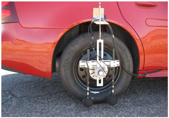
Figure 1. OBSI Equipment Installed on a Test Vehicle
