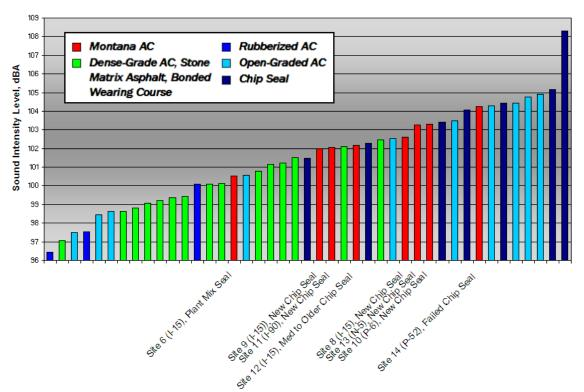
Figure 6. Overall A-Weighted OBSI Levels for AC Pavements, 60 mph
