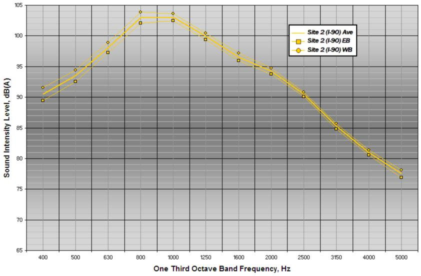
Figure A6. One-Third Octave Band Levels for Site 2 (I-90), Transverse Tine PCC Pavement in EB & WB Directions
