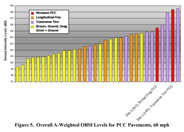
Figure 5. Overall A-Weighted OBSI Levels for PCC Pavements, 60 mph
