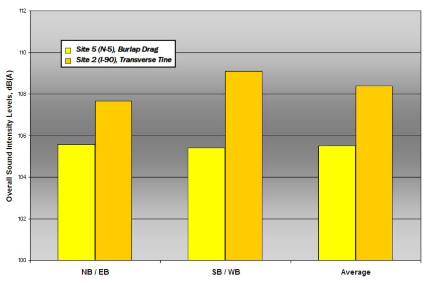
Figure A3. Overall A-Weighted OBSI Levels for PCC Pavements in Each Direction, 60 mph
