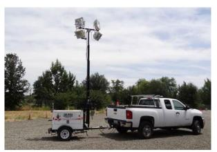
Figure 7. Magnum MLT3060 metal Halide lighting trailer used in the Experimentation.
