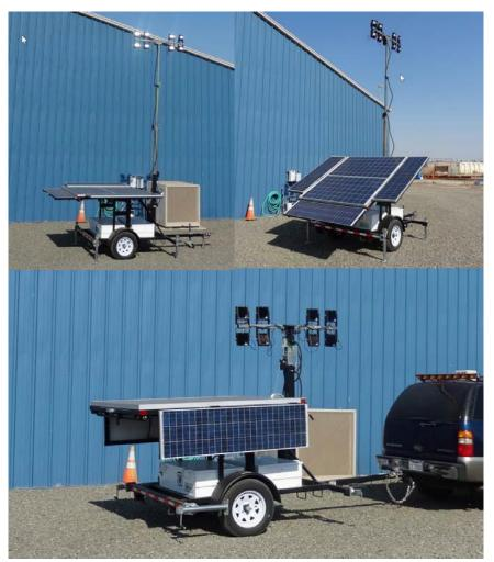
Figure 19. The Solar Light Panels of the Wanco Solar Lighting Trailer.
