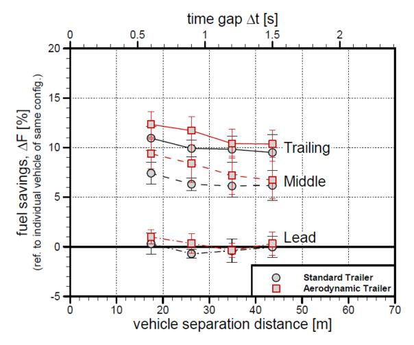
Figure 4. Variation in fuel saving measurements with separation distance for each vehicle in CACC string, fully loaded, 65 mph, (measurements referenced to the *same vehicle configurations* driven individually, without CACC)
