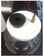
Image 1: Glass jar lid with #8 rubber stopper and air nozzle connector.
