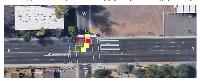
Figure 2.8: Conflict zones of the south-to-west left turning movement at the intersection, where Uber accident occurred.
