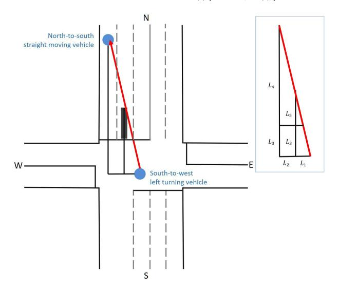
Figure 2.12: Occlusion schematic for the Uber accident scenario.
