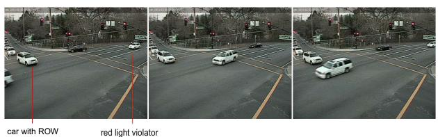
Figure 2.20: Intrusion of red-light violator detected by intersection (source: [15]). Above: picture of a Google AV crash by a red-light violator.
