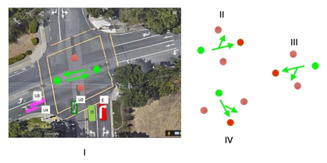
Figure 2.7: The possible signal light configurations (I-IV) compatible with RTOR movement of the ego vehicle.
