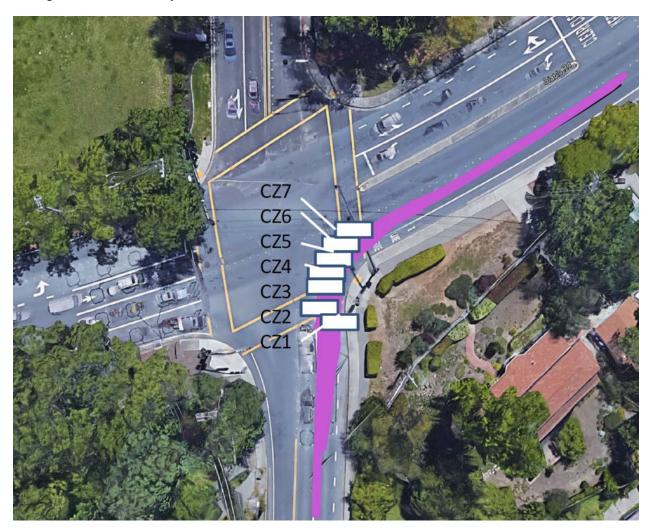
Figure 2.5: The intersection of the seven guideways with the pink guideway yields seven conflict zones, CZ1, ..., CZ7. The conflict zones are shown disjoint for clarity, although in fact they overlap.
