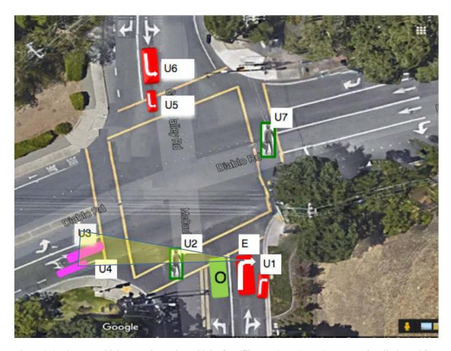
Figure 2.6: The ego vehicle must determine which of conflicts CZ2, CZ3, CZ4, CZ5 can be eliminated from what it sees of the intersection. O obscures the triangular region from the ego vehicle's field of view so it cannot see U2, U3, U4, hence CZ2, CZ3, CZ4 remain.
