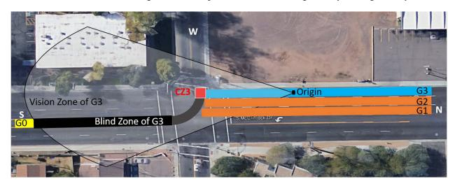
Figure 2.11: Potential blind zone of guideway G3 in guideway G0.
