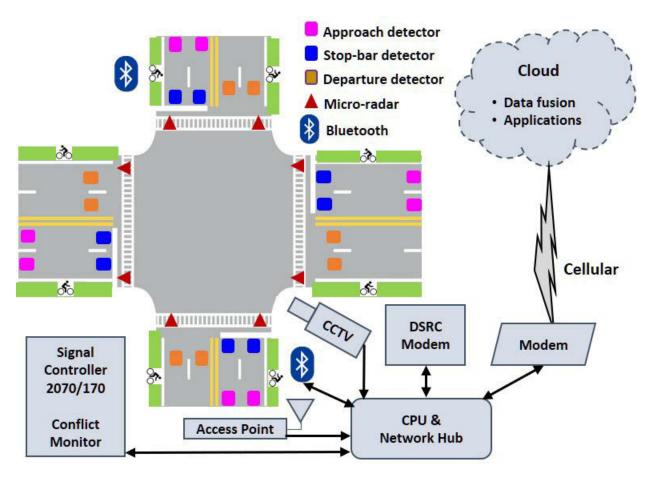
Figure 2.19: Schematic of reference intersection instrumentation.
