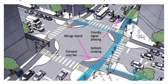
Figure 2.21: Schematic of a protected intersection. Source: [16]
