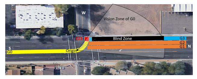
Figure 2.10: Potential blind zone of guideway G0 in guideway G3.
