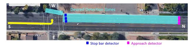
Figure 2.16: Desired detection for the south-to-west left turn movement.
