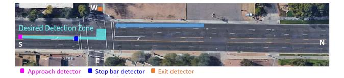
Figure 2.17: Desired detection for the north-to-south through movement.
