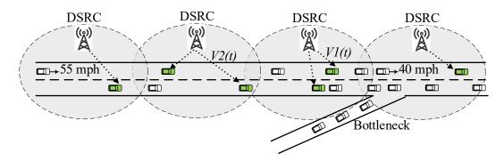
Fig 30. Scenario 2 of I2V Speed Harmonization Application.
