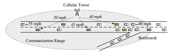
Fig 29. Scenario 1 of I2V Speed Harmonization Application.
