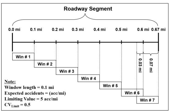
Figure 3: Schematic diagram of the Peak Searching approach
