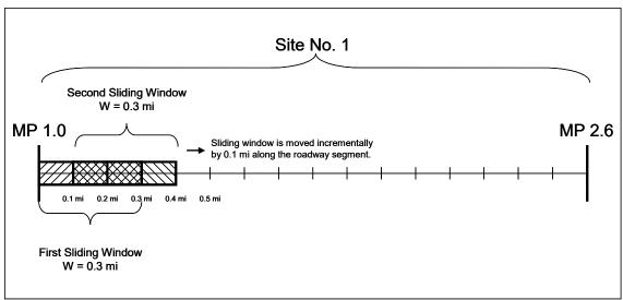
Figure 2: Schematic diagram of the Sliding Window approach
