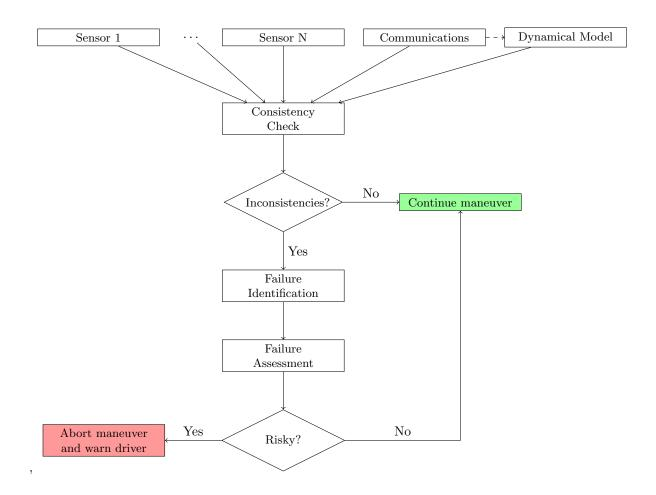
Figure 16: Flowchart of verification procedure with N independent sensors.
