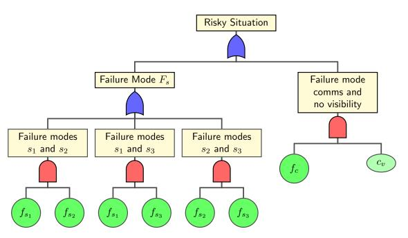
Figure 18: Fault Tree for gap verification
