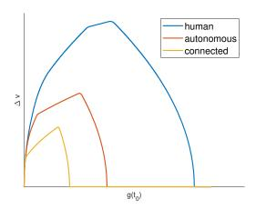
Figure 3: Severity as a function of the initial gap for the different driver types described in [6].
