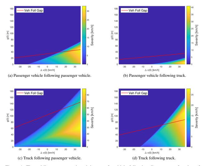
Figure 4: The red line represents the minimum safe vehicle following distance as a function of the relative velocity The color map indicates the severity, as computed from Eq. (4), of a collision under the described worst-case scenario for each combination of initial gap and velocity.
