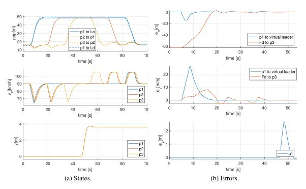
Figure 23: Vehicle states (a) and relevant errors (b) for platoon lane change with the Synchronous strategy and zero initial relative velocity between lanes. Plots on the left from top to bottom show inter-vehicle gaps, longitudinal velocity and lateral position. Plots on the right from top to bottom show headway, velocity and lateral errors.
