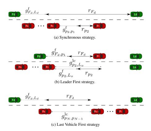
Figure 26: Examples of reserved space  $r_k(t)$  for different vehicles and in different traffic configurations.
