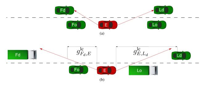
Figure 17: Ego vehicle visibility of vehicles on the destination. On top, all vehicle are visible. At the bottom, a configuration where follower and leader on the origin lane "hide" their counterparts at the destination lane. Red arrows indicate E's measurements and black arrows show the safe lane change gaps.
