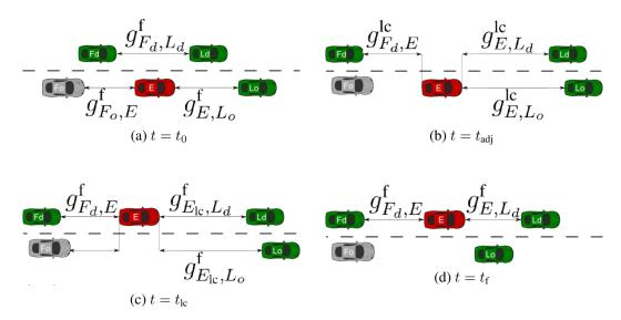
Figure 19: Examples of vehicle configurations at the different lane change phases. The red egovehicle must monitor the gaps to the three green vehicles  $F_d$ ,  $L_d$  and  $L_o$ . The dependence of safe gaps on time is omitted to improve figure clarity.
