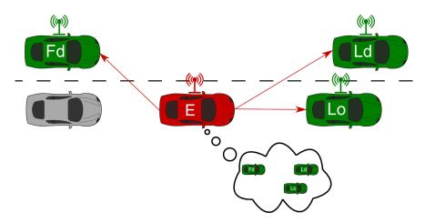
Figure 15: The ego vehicle monitors its surrounding vehicles. Arrows indicate sensor measurements, an antenna indicates the vehicle is communicating, and the thought bubble represents E's internal model of the others.
