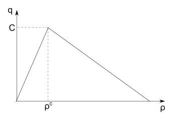
Figure 29: Example of typical fundamental diagram.
