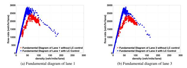
Figure 30: Fundamental diagrams with (blue) and without (red) lane change control for the remaining open lanes.
