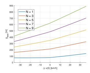
Figure 13: Minimum gap at the adjacent lane as a function of the relative velocity between lanes for different number of vehicles in the platoon.
