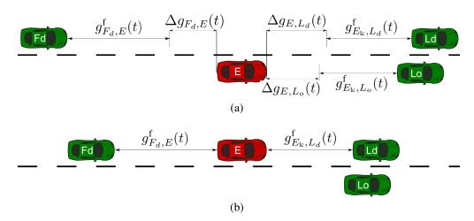
Figure 1: In (a), minimum safe lane change gaps that must be created before the maneuver can start. In (b), expected distances right after the maneuver is completed.
