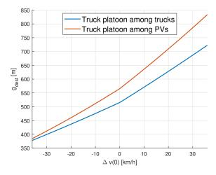
Figure 14: Minimum gap at the adjacent lane for a five vehicle truck platoon as a function of the relative velocity between lanes. In blue, the truck platoon merges between trucks and, in red, it merges between passenger vehicles.
