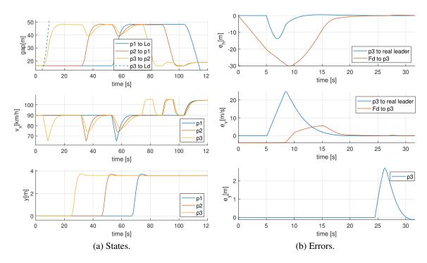
Figure 25: Vehicle states (a) and relevant errors (b) for platoon lane change with the Last Vehicle First strategy and positive initial relative velocity between lanes. Plots on the left from top to bottom show inter-vehicle gaps, longitudinal velocity and lateral position. Plots on the right from top to bottom show headway, velocity and lateral errors.
