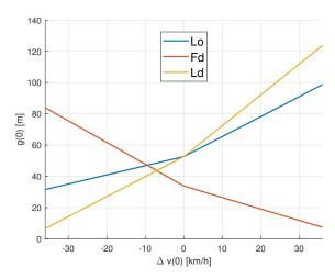
Figure 5: Minimum lane change safe spacing from  $L_o$  (blue),  $F_d$  (red) and  $L_d$  (yellow) as a function of relative velocity.
