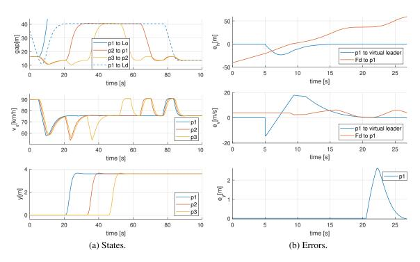
Figure 24: Vehicle states (a) and relevant errors (b) for platoon lane change with the Leader First strategy and negative initial relative velocity between lanes. Plots on the left from top to bottom show inter-vehicle gaps, longitudinal velocity and lateral position. Plots on the right from top to bottom show headway, velocity and lateral errors.
