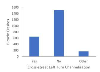
Figure 3-14. Bicycle intersection crashes by left turn channelization on cross-street (2013-2017)
