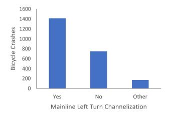
Figure 3-13. Bicycle intersection crashes by left turn channelization on mainline (2013-2017)
