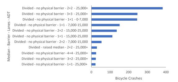
Figure 3-24. Bicycle highway crashes by median type, number of lanes (left & right) and vehicular traffic volumes (2013-2017)
