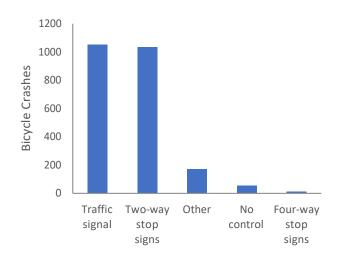
Figure 3-11. Bicycle intersection crashes by type of traffic control (2013-2017)
