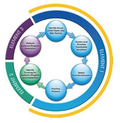
Figure 3-1. FHWA's Systemic Safety Project Selection Tool. Element 1: The Systemic Safety Planning Process (from FHWA 2013)
