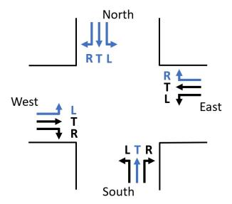
Figure 4-2. Intersection turning movements with north approach counts in blue
