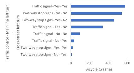
*Figure 3-15. Bicycle intersection crashes by type of traffic control and left turn channelization (mainline & cross-street) (2013-2017)*
