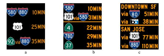
Figure 18. Travel Time and Up to Six Lines Messages
