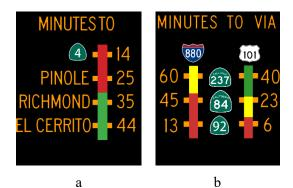
Figure 6. Examples of Single-link GRIP and Dual-link GRIP
