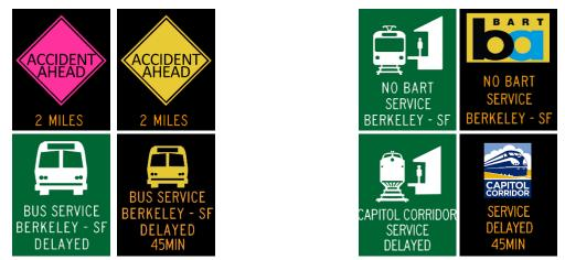
Figure 15. Proposed Design for the Four Special Messages
