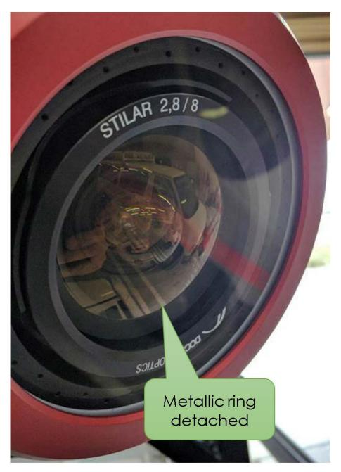
Figure 2.5: Close-up view of VMX-1HA Camera 2 lens. The metallic ring detached from the lens and contacted the camera housing glass cover.
