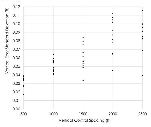
Figure 6.11: Left laser vertical (Z-direction) error standard devation of each pass traveling on left lane at various vertical control registration spacings
