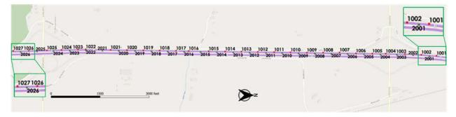
Figure 6.3: Aerial view of GTPG site MTLS targets overlaid on Microsoft Bing Maps. The red squares with numbers 10xx mark the location of MTLS targets on the shoulder. The green squares with numbers 20xx mark the location of MTLS targets on the median.
