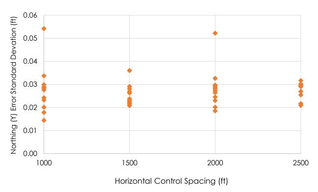
Figure 6.9: Left laser Northing (Y) standard devation of each pass traveling on number 1 lane at various registration control spacings
