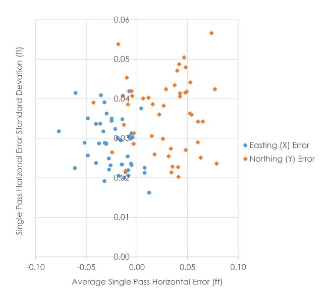
Figure 6.6: Average horizontal (Easting X- and Northing Y-direction) error vs. horizontal error standard devation for left and right laser data of each pass in all four sessions
