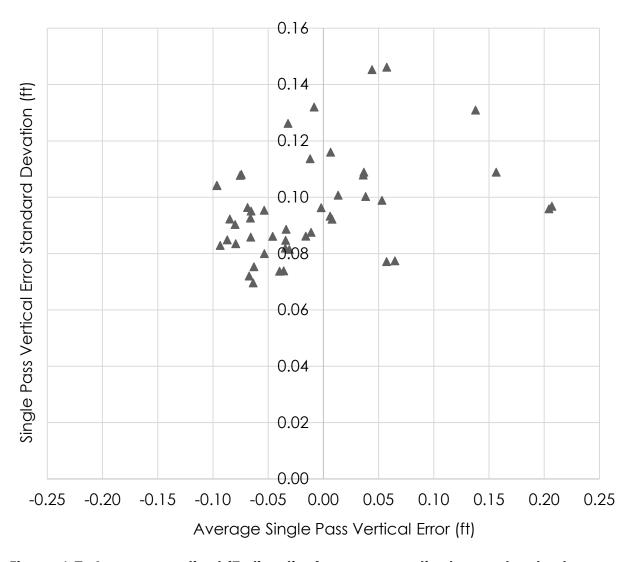
Figure 6.7: Average vertical (Z-direction) error vs. vertical error standard devation for left and right laser data of each pass in all four sessions
