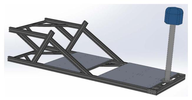
Figure 5.2: CAD model of the standing platform with Ladybug 5+ camera mount and cover
