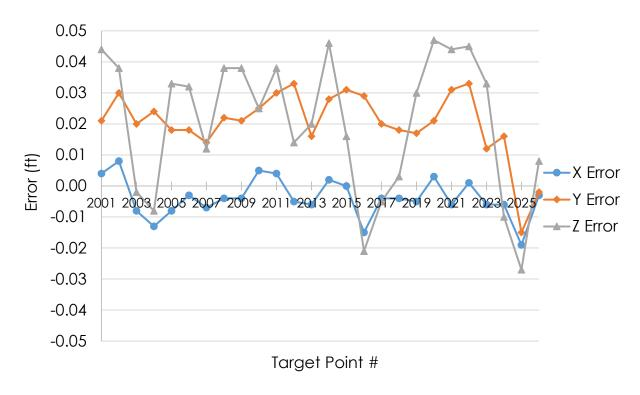
Figure 6.5: Example of position errors vs. MTLS targets before registration (06/12/2019 pass #5)
