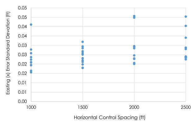
Figure 6.8: Left laser Easting (X) error standard devation of each pass traveling on number 1 lane at various registration control spacings
