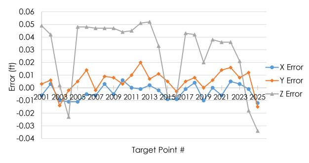
Figure 6.4: Example of position errors vs. MTLS targets before registration (06/06/2019 pass #4)
