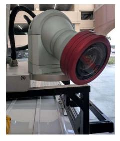
Figure 2.4: VMX-1HA Camera 2 mounted on the rear passenger side of the vehicle
