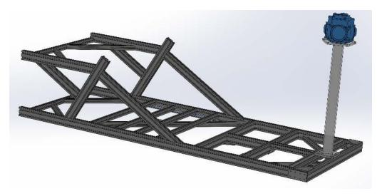
Figure 5.3: CAD model of the standing platform and Ladybug 5+ camera mount with standing plate and camera cover removed
