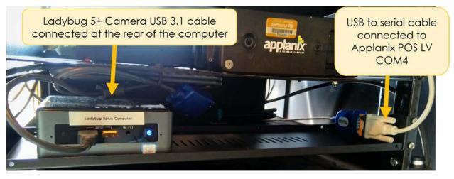
Figure 5.6: Ladybug 5+ data collection computer setup
