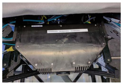
Figure 2.1: Housing for three MX8 front cameras
