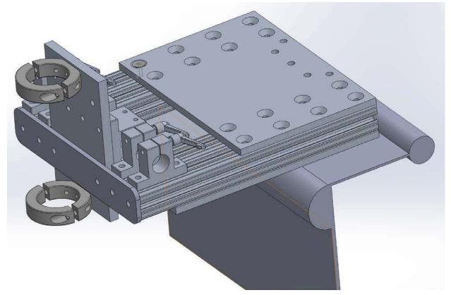
Figure 3.13: Sensor mount CAD model
