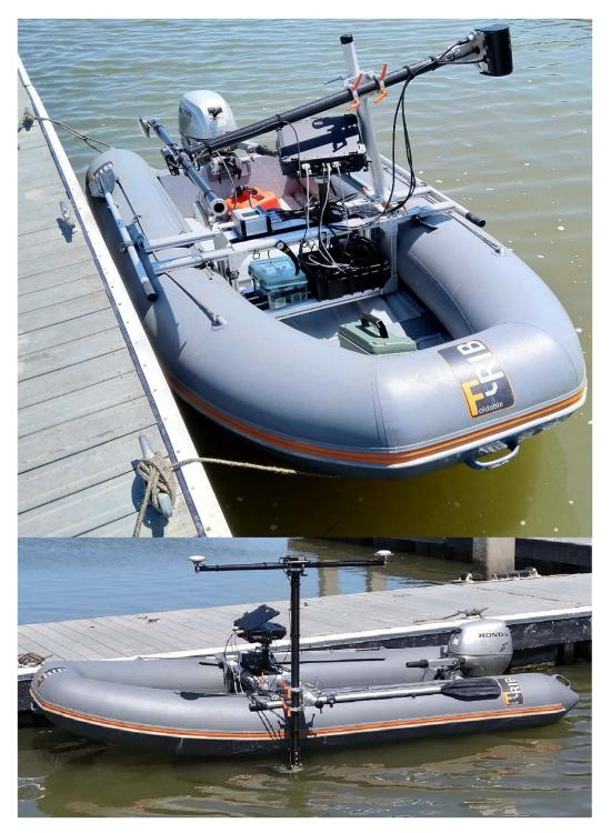
Figure 3.12: PicoMBES testing on Caltrans boat at Napa River (05/22/2020). The top photograph shows the sensor mask pivoted up so that the PicoMBES sensor is out of the water (transit configuration).
