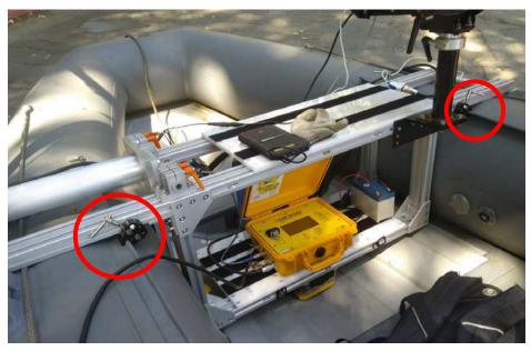
Figure 3.10: Component mounting platform secured in the Caltrans foldable boat with four clamps. Two of the clamps are visible and highlighted by red circles.
