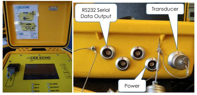
Figure 3.17: CEE Echo computer. Right image shows the RS232 serial port connection location.
