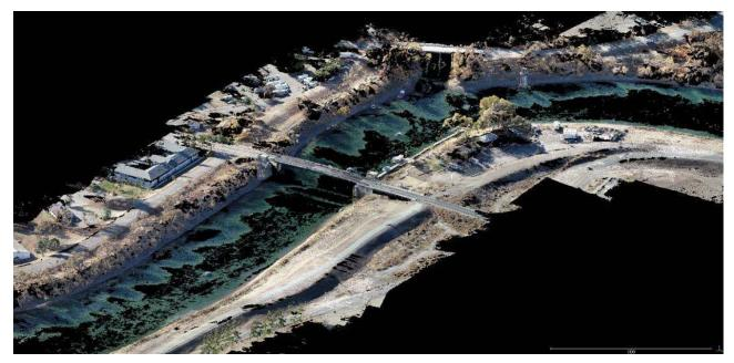
Figure 4.6: SR113 pilot study site point cloud (64 million points) created by WebODM software using 679 aerial images
