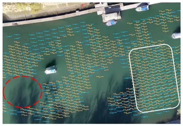
Figure 4.11: RIVeR LSPIV result overlaid on georeferenced orthophoto in QGIS. Area with good natural tracers is highlighted by a white rectangle, and area with poor/no natural tracers is highlighted by a red circle.
