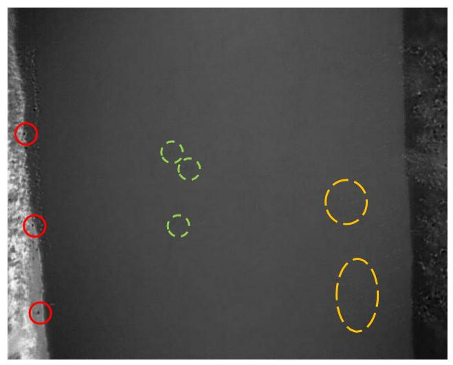
Figure 4.14: Example LSPIV IR video capture frame. Area with good, natural seeding is highlighted by a yellow dashed line. Red circles highlight the GCP targets. Green circles highlight artificial seeding using ice cubes.
