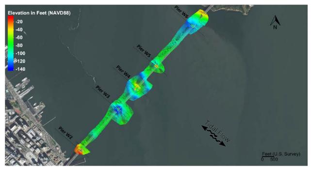
Figure 3.24: Bathymetric survey result of San Francisco-Oakland Bay Bridge, CA
