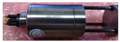
Figure 2.5: Valeport sound velocity sensor, model: UltraSV and S/N: 66056
