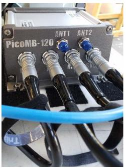
Figure 3.16: PicoMBES 120 system control box
