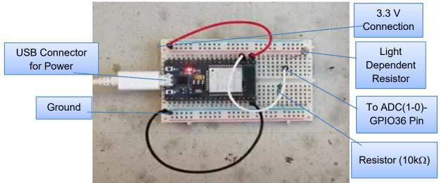
Figure 2: ESP32 Circuit Connection
