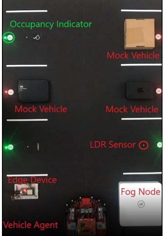
Figure 7: Hardware-in-the-loop simulation
