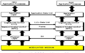
Figure 10: DSRC architecture [1]
