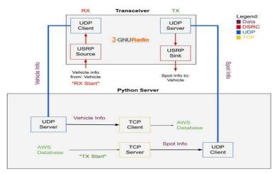
Figure 19: Communication Diagram (Fog Node)
