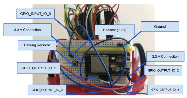
Figure 8: TI robotics vehicle attached with ESP32 for wireless capabilities
