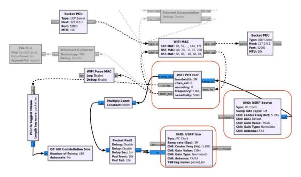
Figure 17: USRP Expanded View (GNU Radio Blocks)
