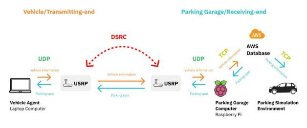
Figure 15: Hardware Diagram
