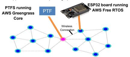
Figure 3: Wireless Sensor Network Design. Currently a star topology between the PTFS and one ESP32 board which can be scaled to include further boards in an XMesh configuration
