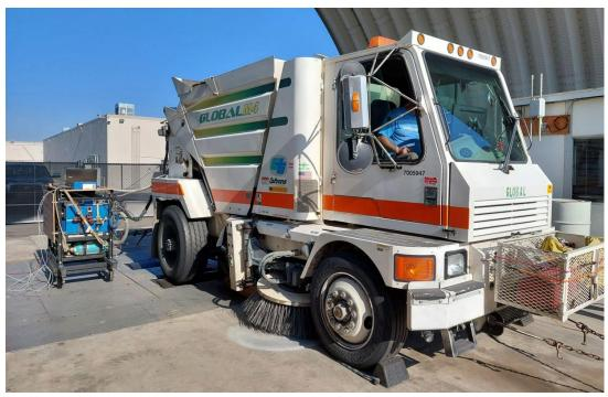
Figure 6-1 Chassis dynamometer test set up
