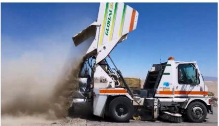
Figure 5-4 Rear dumping event with PEMS equipment installed.
