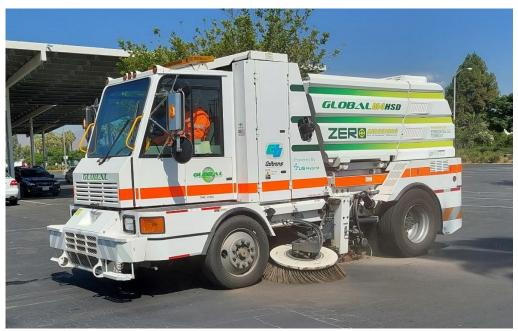
Figure 3-5 Hydrogen fuel cell electric street sweeper
