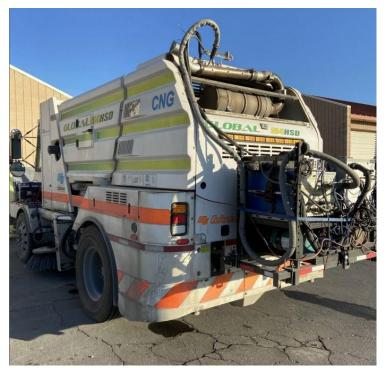
Figure 5-1 PEMS unit mounted to rear of HSD street sweeper
