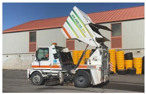
Figure 3-3 Global M4 rear dump street sweeper
