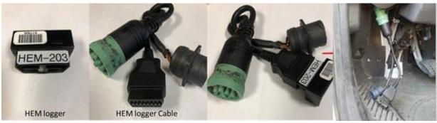
Figure 4-1. HEM data logger and installation
