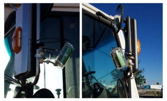
Figure 5-5 Time-lapse cameras mounted for PEMS testing
