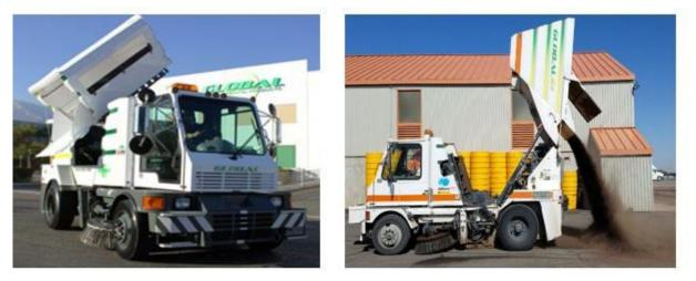
Figure 5-3 a) Global M4HSD high-side dump sweeper and, b) Global M4 rear dump sweeper
