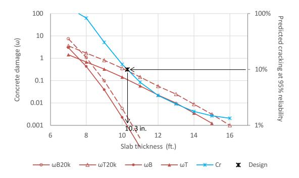
Figure 3.1: Illustration of approach for determining slab thickness.
