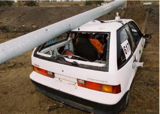
Figure 2-65. Damage to Rear Roof
