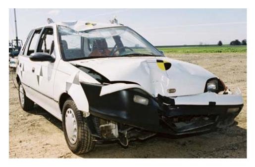
Figure 2-37. Test Vehicle After Test 618
