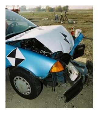
Figure 2-9. Test Vehicle After Test 611
