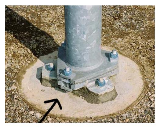
Figure 2-38. Close-Up View of Type 30/31 Slip-Base Used in Test 618 (Arrow Indicates Direction of Vehicular Impact)
