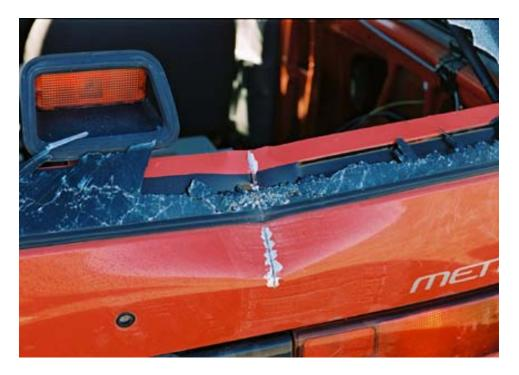
Figure 2-27. Lower Section of Hatchback of Test Vehicle After Test 614
