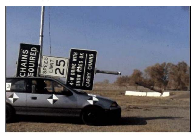
Figure 2-21. Chain Control Sign Penetration into Windshield (Test 613)
