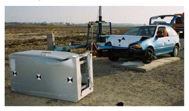
Figure 2-12. Controller Cabinet Test Article and Vehicle After Test 611
