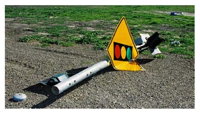
Figure 2-51. Test Article After Test 616
