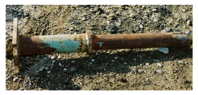
Figure 2-19. Breakaway Base From Test Article After Test 613
