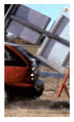
Figure 2-32. Chain Control Sign Penetration into Rear Window – Test 614
