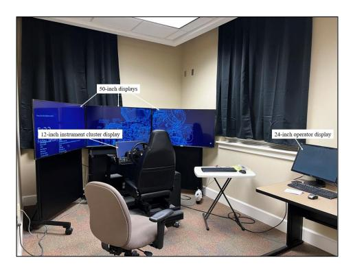
Figure 3.1 Driving Simulator Displays
