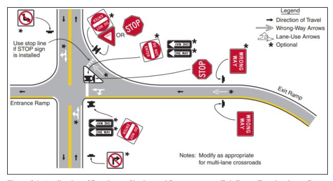
Figure 2.1. Application of Regulatory Signing and Pavement at an Exit Ramp Termination to Deter Wrong-Way Entry (MUTCD 2009)
