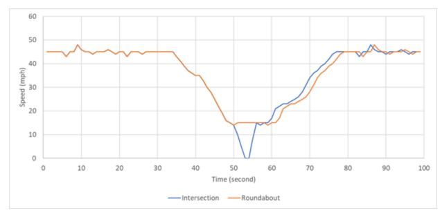
Figure 4. Drive cycle used in MOVES.
