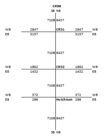
Figure 5. ADT data for the three intersection (NB-Northbound; SB – Southbound; EB – Eastbound; WB – Westbound)
