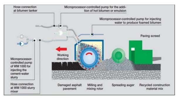
Figure 8. FDR equipment (Wirtgen, 2012).
