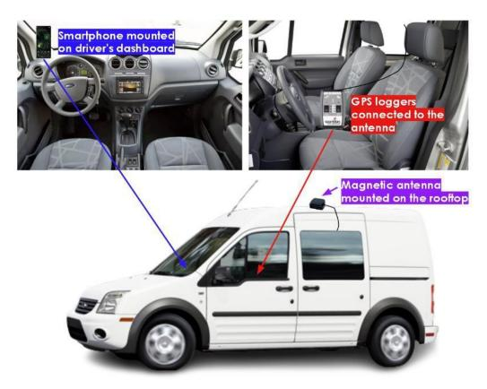
Figure 3.1: Equipment setup
