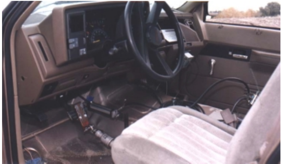
Figure 2-29 Post Impact Interior View of Vehicle 545
