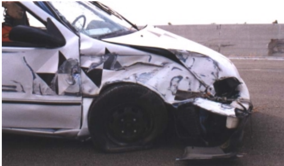
Figure 2-17 Close up of Passenger Side Front Damage, Vehicle 544
