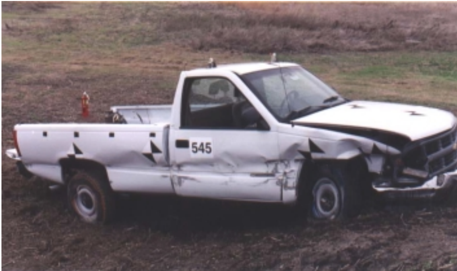
Figure 2-27 Post Impact Side of Test Vehicle 545
