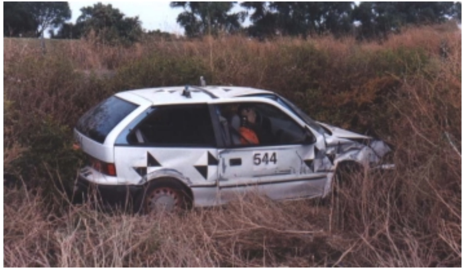
Figure 2-16 Post Impact Side View of Vehicle 544
