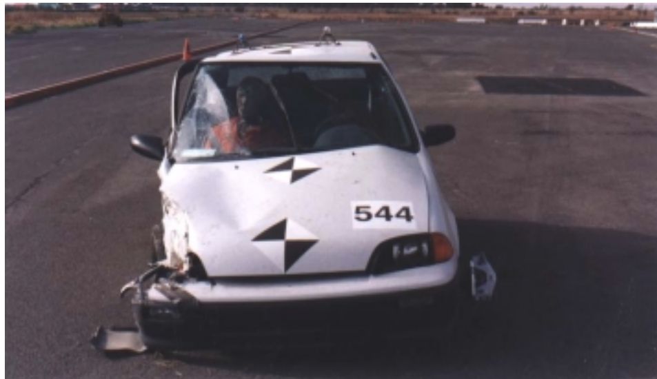
Figure 2-18 Post Impact Front View, Vehicle 544
