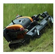
Figure 20. RoboFlail plus RC Tool-Carrier Tractor
