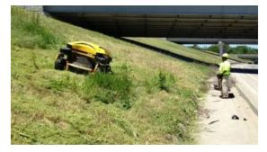
Figure 4. Illinois TA Operating ILD02 RC Mower
