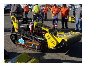
Figure 14. Caltrans Traxx-RF RC Tool-Carrier Tractor
