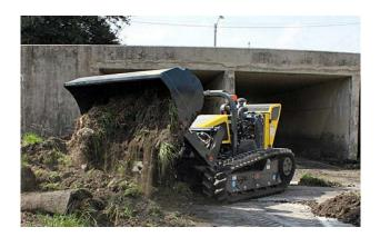
Figure 15. RoboGreen RC Tool-Carrier Tractor Equipped with Bucket
